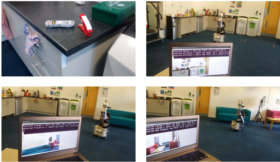
Figure 6. Object detection. The three tagged objects (kitchen table, remote control, stapler) are shown on the top-left. The remaining figures show the moment in which the objects were correctly detected by the robot navigating in a simulated domestic environment. The name, RSSI and Phase of the objects are printed on the laptop screen at the bottom of each figure.
