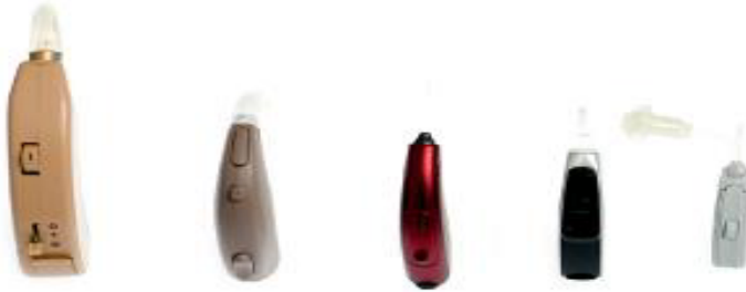
Figure 1. Miniaturization from an analogue hearing aid (on the left) to a modern digital one (on the right) 2
