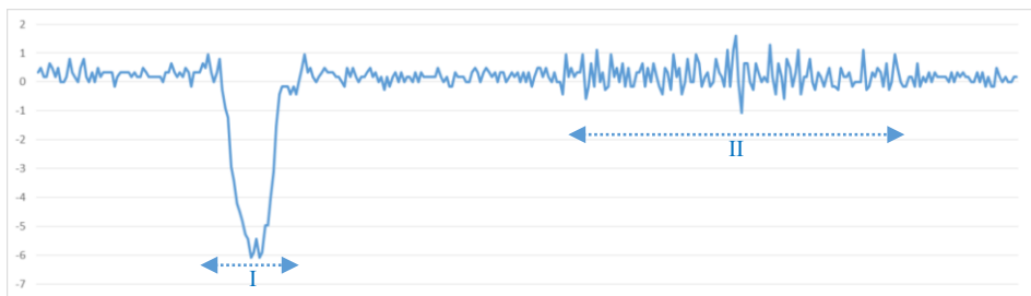
Figure 2. Scaled and normalized accelerometer data. The roman number I and II denote movements.
