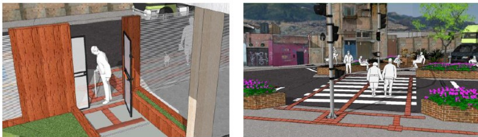
Figure 4. Idea: A parallel comparison of two important modes of perception. At the entrance gate, there are coloured bars. At the street, planters and tactile stripes make crosswalk safe.
