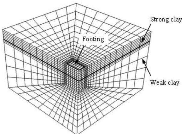
Figure 3. Finite element mesh for rectangular footing  $L/B = 2.0$ .
