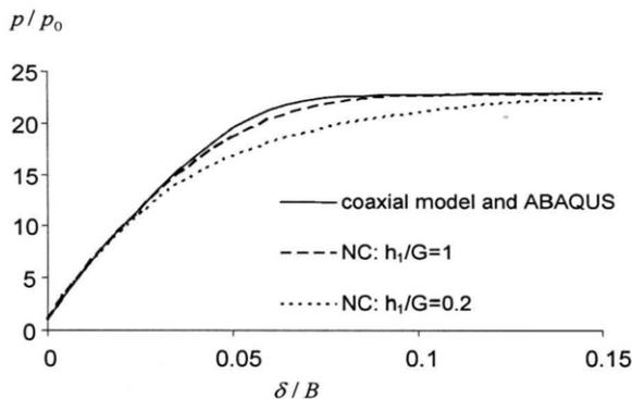
Figure 7. Footing settlement predictions under uniform loading using Rudnicki & Rice's non-coaxial model with different values of  $h_1/G$
