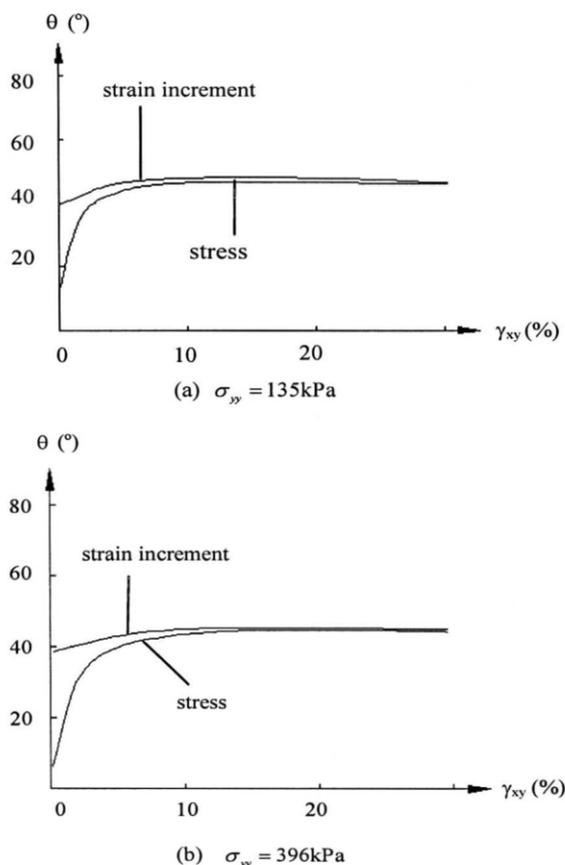
Figure 1. Experimental curves of showing principal stress and strain increment rotations against shear strain during simple shear test [After Roscoe (1970)]
