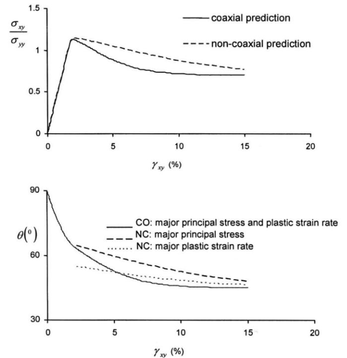
Figure 5. The evolutions of shear stress ratio and orientation of major principal stress and plastic strain rates in a simple shear of sand with  $K_0$  equal to 3.0 using Rudnicki & Rice's theory
