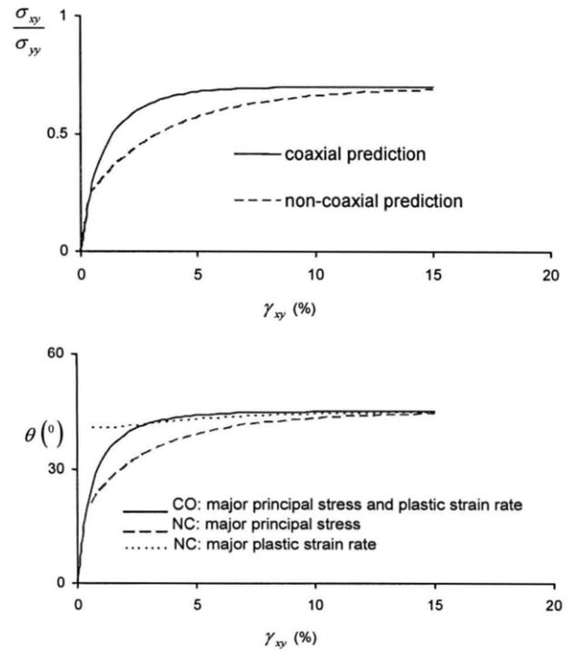
Figure 4. The evolutions of shear stress ratio and orientation of major principal stress and plastic strain rates in a simple shear of sand with  $K_0$  equal to 0.4 using Rudnicki & Rice's theory
