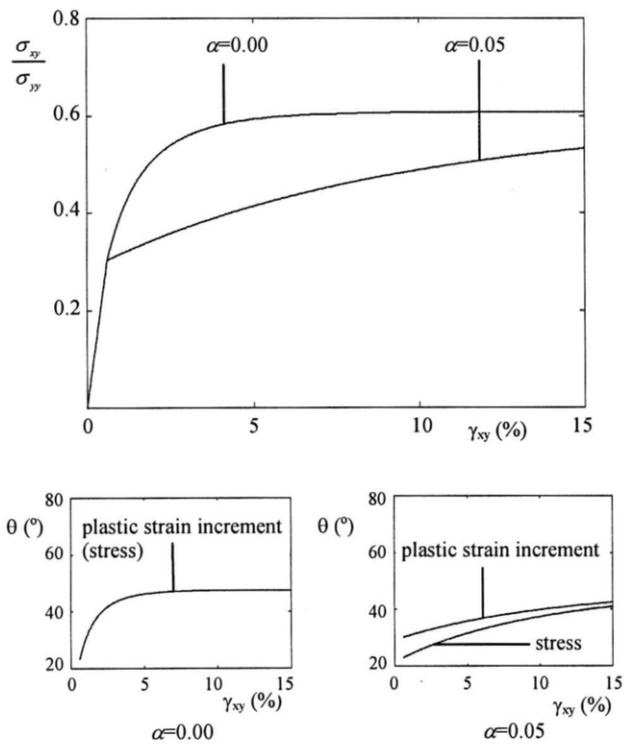
Figure 2. The evolutions of shear stress ratio and orientation of major principal stress and plastic strain rates in a simple shear of sand with  $K_0$  equal to 0.4 using Harris' theory
