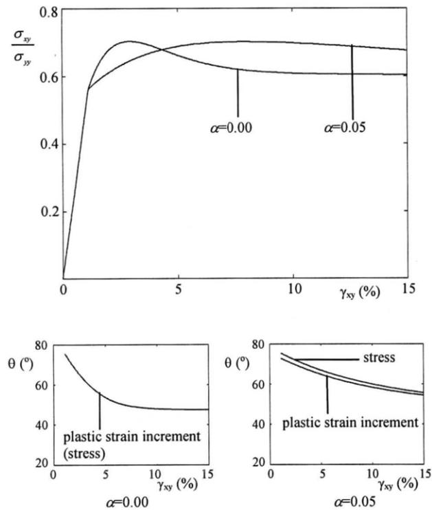
Figure 3. The evolutions of shear stress ratio and orientation of major principal stress and plastic strain rates in a simple shear of sand with  $K_0$  equal to 3.0 using Harris' theory
