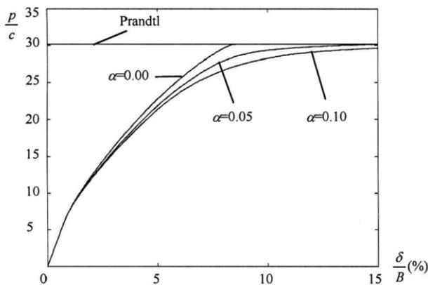
Figure 6. Footing settlement predictions under uniform loading using Harris' non-coaxial model with different values of  $\alpha$
