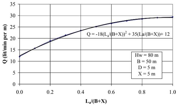
Figure 4. Effect of Ancillary Drain on Discharge Results
