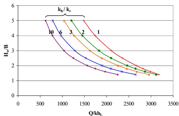
Figure 7. Design Chart: Effect of Anisotropic Permeability on Discharge  $D/B = 0.2$ ;  $X/D = 1$
