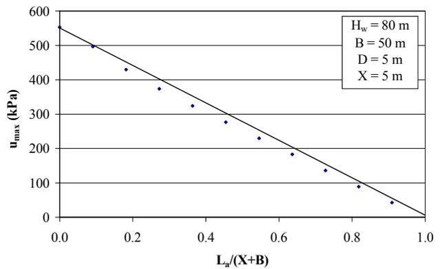
Figure 2. Effects of Ancillary Drain on Pore water Pressure Measurements
