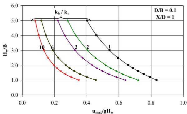
Figure 5. Design Chart for Pore Pressure Measurements for Anisotropic Fill Material:  $D/B = 0.1$ ;  $X/D = 1$
