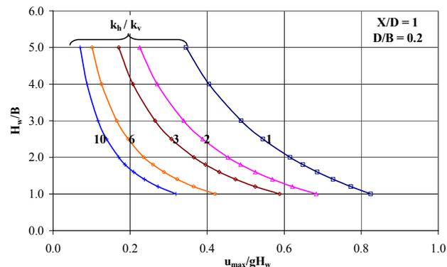
Figure 6. Design Chart for Pore Pressure Measurements for Anisotropic Fill Material:  $D/B = 0.2$ ;  $X/D = 1$
