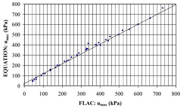
Figure 3. Comparison between Maximum Pore Pressures Obtained from FLAC and those Calculated using Equation 2.
