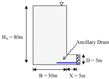
Figure 1. Geometry of Stope with Ancillary Drainage
