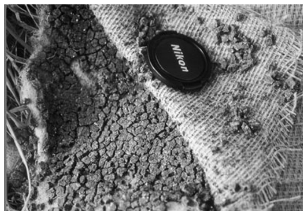
Figure 6. Photograph of desiccated bentonite in a GCL exhumed from a cap in southwestern Wisconsin (from Benson, 2002).
