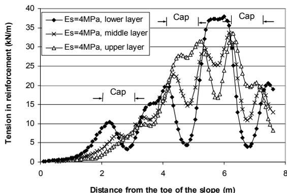
Figure 6. Tension distribution in reinforcement in the x-direction
