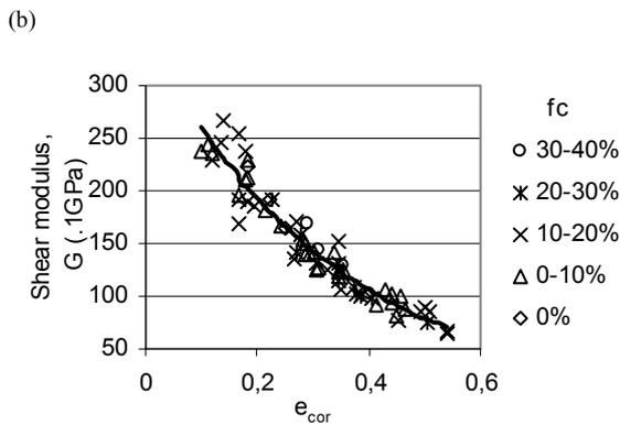
Figure 8 Shear modulus versus void ratio (a) and corrected void ratio (b) for different fines content  $f_c$ , confining pressure 30 MPa (data from Han et al. 1986)
