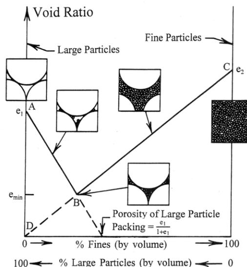
Figure 1 Binary packing with different fines content (Lade et al. 1998)
