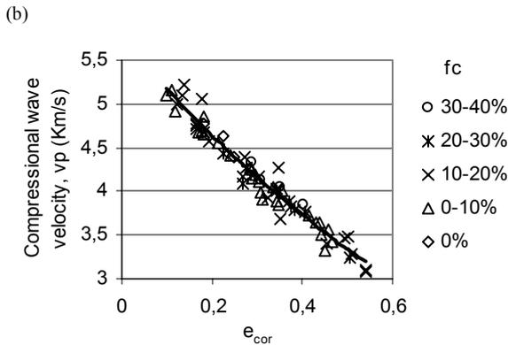
Figure 5 Compressional wave velocity versus void ratio (a) and corrected void ratio (b) for different fines content  $f_c$ , confining pressure 30 MPa (data from Han et al. 1986)
