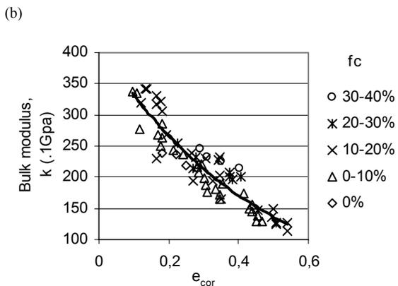
Figure 7 Bulk modulus versus void ratio (a) and corrected void ratio (b) for different fines content  $f_c$ , confining pressure 30 MPa (data from Han et al. 1986)
