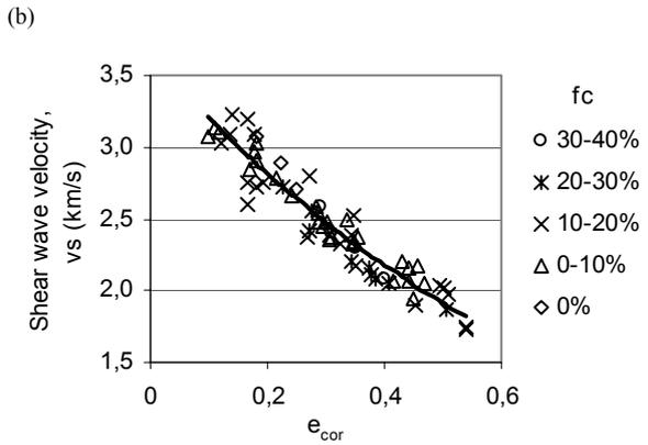
Figure 6 Shear wave velocity versus void ratio (a) and corrected void ratio (b) for different fines content  $f_c$ , confining pressure 30 MPa (data from Han et al. 1986)
