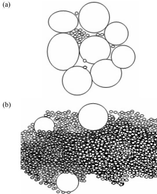
Figure 3 Sand with low (a) and high fines content (b)
