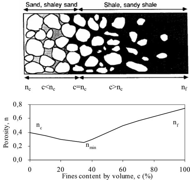
Figure 2 Ideal packing model (modified from Marion et al. 1992 and Koltermann and Gorelick, 1995)
