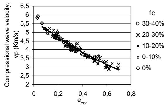
Figure 10 Compressional wave velocity versus void ratio (a) and corrected void ratio (b) for different fines content  $f_c$ , confining pressure 40 MPa (data from Han et al. 1986 and Klimentos and McCann 1990)
