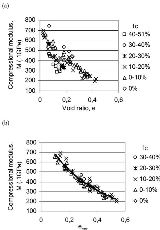
Figure 9 Compressional modulus versus void ratio (a) and corrected void ratio (b) for different fines content  $f_c$ , confining pressure 30 MPa (data from Han et al. 1986)
