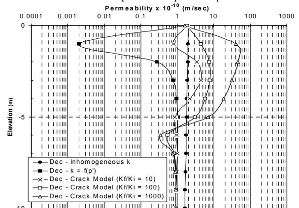
Figure 7 Influence of cracked permeability model on magnitude of permeability at the end of December.
