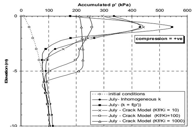
Figure 3 Influence of cracked permeability model on accumulated  $p'$  at the end of July.
