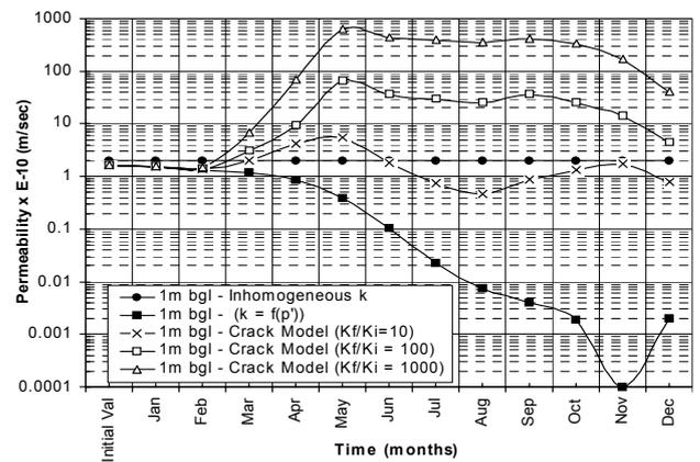
Figure 10 Influence of  $k_f/k_i$  ratio on permeability at 1m bgl.
