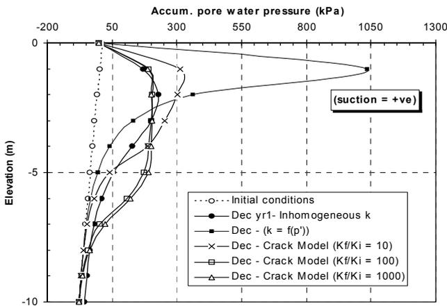
Figure 8 Influence of cracked permeability model on accumulated pore water pressure at the end of December.
