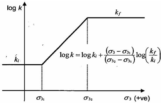
Figure 1 Variation of mass permeability with  $\sigma_3$  in the new model.
