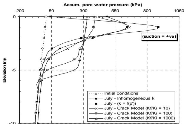
Figure 5 Influence of cracked permeability model on accumulated pore water pressure at the end of July.
