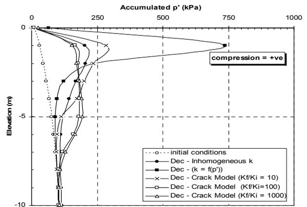
Figure 6 Influence of cracked permeability model on accumulated  $p'$  at the end of December.
