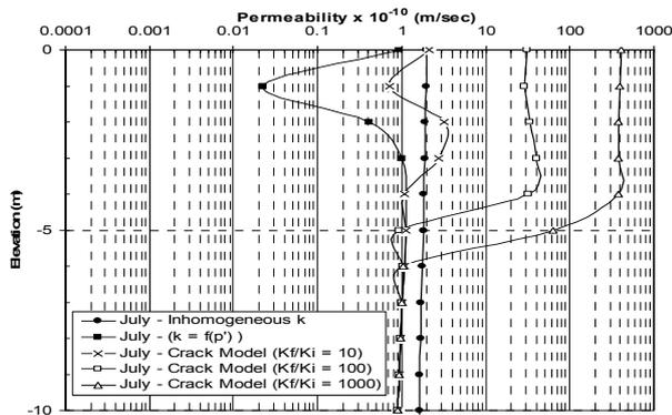
Figure 4 Influence of  $k_f/k_i$  ratio on magnitude of permeability at the end of July.
