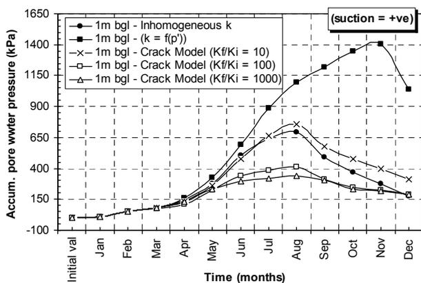
Figure 9 Influence of cracked permeability model on accumulated pore water pressure at 1m bgl.
