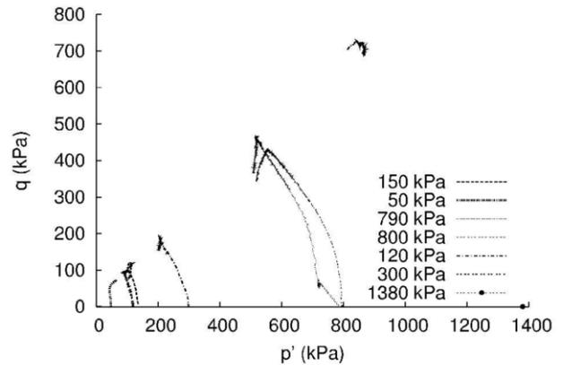
Figure 6. Stress paths of the triaxial tests.
