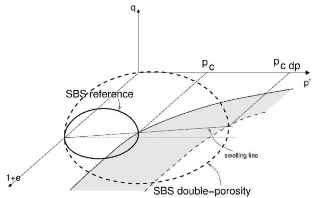
Figure 4. SBS of double-porosity and reference materials
