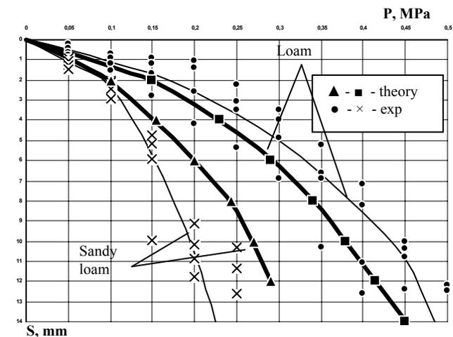
Figure 1. Diagrams of the plate settlement from load.
