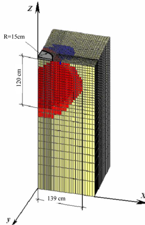
Figure 3. Zones of limit condition of the soil ground (loam sandy).
