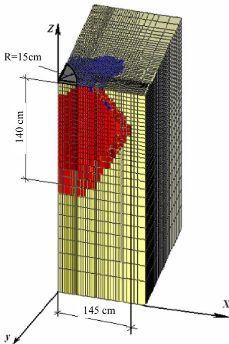
Figure 2. Zones of limit condition of the soil ground (loam).
