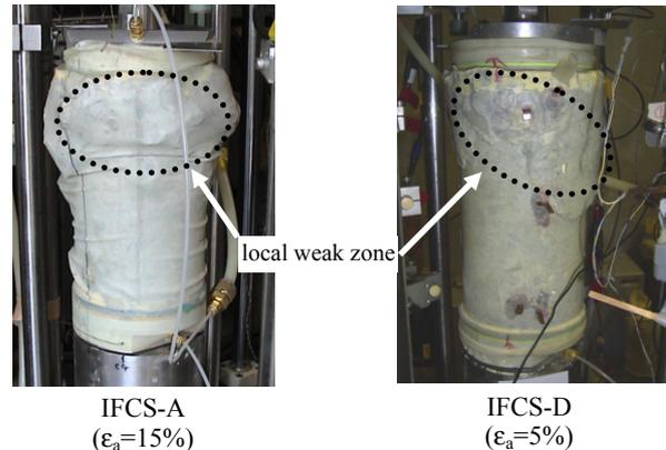
Figure 7. Deformed specimen after peak state
