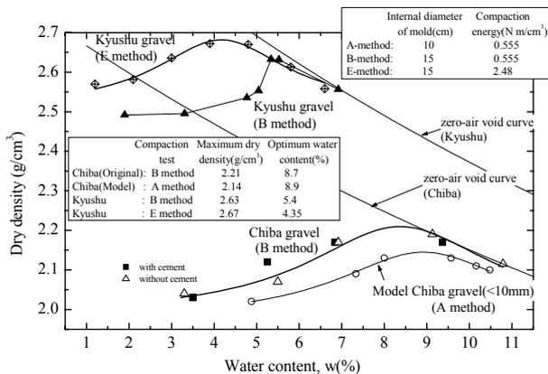
Figure 2. Compaction curves of Chiba gravel and Kyushu gravel
