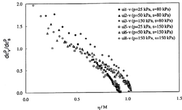
Figure 2. Stress-dilatancy relationship for specimens of decomposed volcanic soil under constant water content stress path (after Chiu, 2001).
