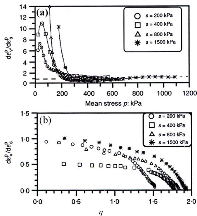
Figure 1. Effect of suction on dilatancy of silt under (a) constant stress ratio ( $\eta = 1$ ) and (b) constant cell pressure ( $\sigma_3 = 200\text{kPa}$ ) (after Cui & Delage, 1996).
