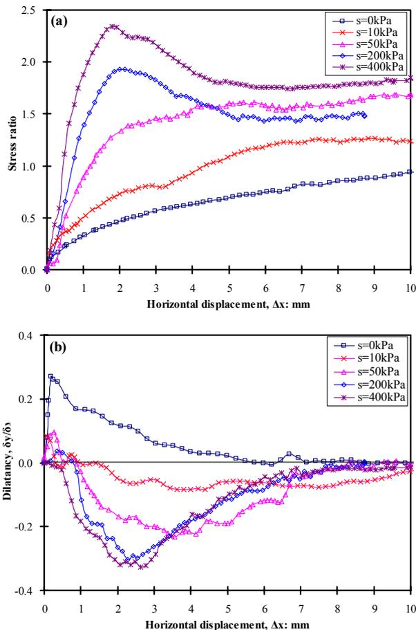
Figure 5. Evolution of stress ratio and dilatancy of CDG subjected to shear under different controlled suctions.
