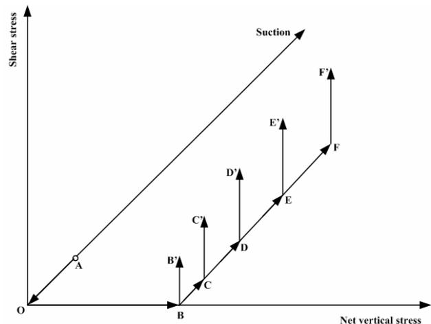
Figure 4. Stress paths in direct shear box tests.
