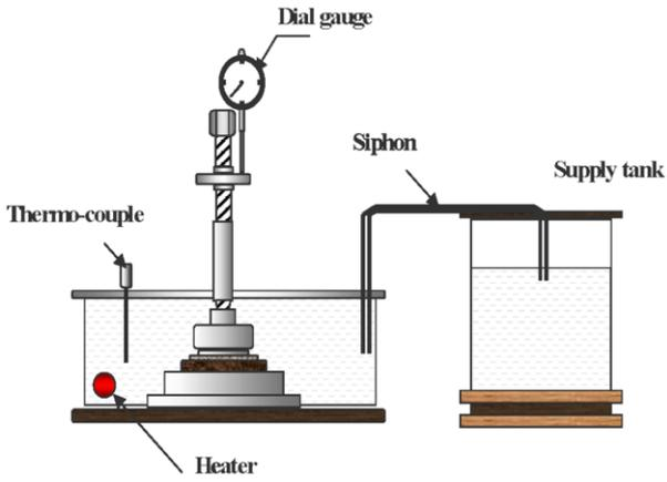
Fig. 1 Modified 1-D oedometer test
