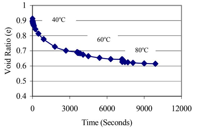
Fig. 4 Volume change during thermal loading (300 kPa)
