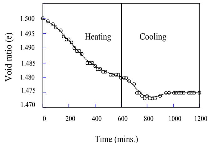
Fig. 8 Results from Heating of Clay (70°C) and subsequent cooling down to room temperature (35°C) under 300 kPa normal pressure.
