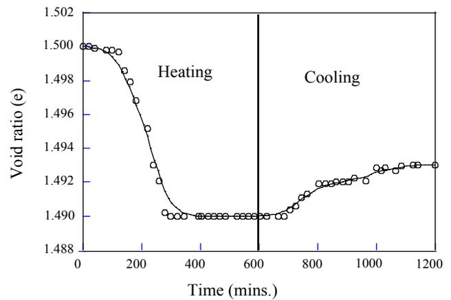
Fig. 7 Results from Heating of Clay (80°C) and subsequent cooling down to room temperature (35°C) under 150 kPa normal pressure.
