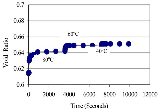
Fig. 5 Volume change during thermal unloading (Unloading under 300 kPa)
