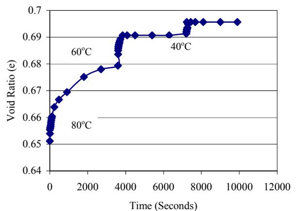
Fig. 6 Volume change during thermal unloading (Unloading from 300 kPa to 150 kPa)
