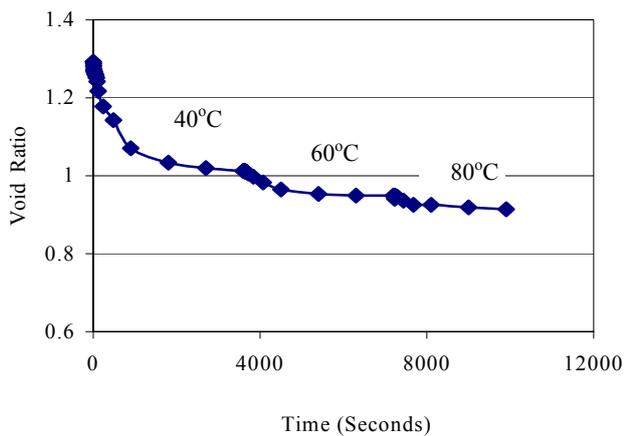
Fig. 3 Volume change during thermal loading (75 kPa-150 kPa)
