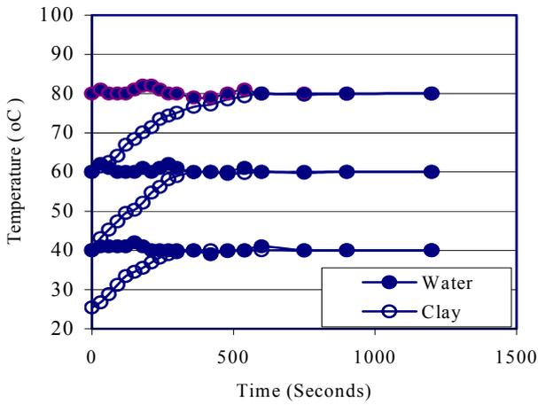
Fig. 2 Temperature build-up in specimen and water bath
