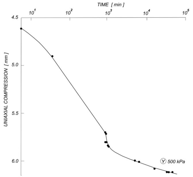
Figure 7. Garlandlike creep with two-layered specimen (upper layer – dry granulated clay, lower layer – wet granulated clay) – perfect garland
