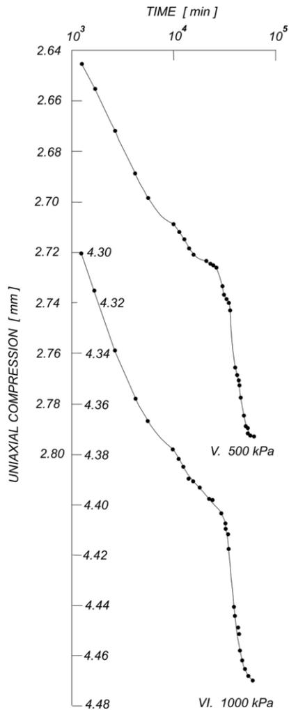
Figure 5. Tests V, VI – enlarged for  $t > 10^3$  min
