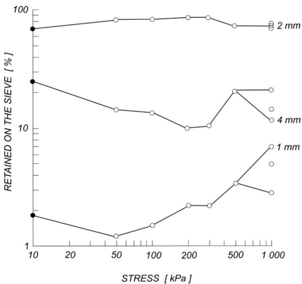
Figure 10. Clayey grains fractions on sieves 1, 2 and 4 mm
