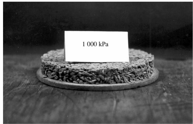
Figure 11. Lateral view of the specimen of granulated clay after being loaded by 1000 kPa
