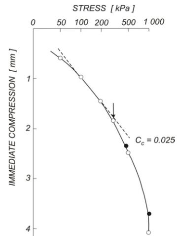
Figure 3. Immediate compression curve of granulated clay. Full circles – repeated tests.
