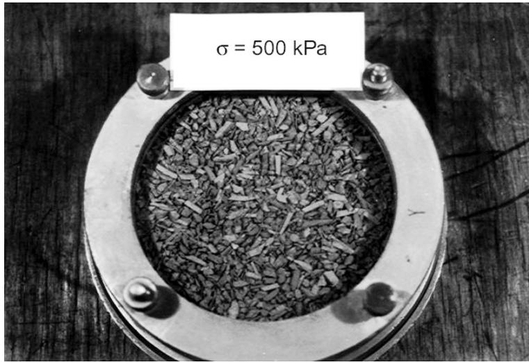
Figure 1. Oedometer ring after the test with 500 kPa
