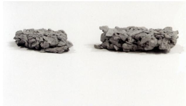
Figure 12. Aggregates of clayey grains after the application of the load 1000 kPa
