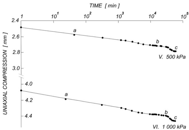
Figure 2. Oedometer creep curves of dry granulated loose Neogene clay at different stress levels
