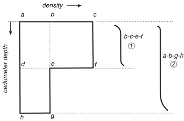
Figure 9. Illustration of the nonhomogeneity effect in Fig. 8 due to the variable density of the specimen
