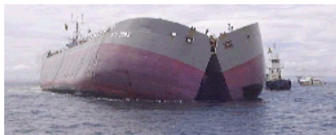
Figure 18. Soil dumping by hopper barge
