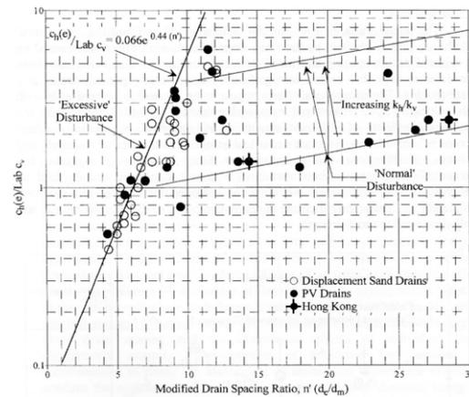
Figure 5. Effect of disturbance due to PV drain installation on consolidation properties of soft clays (Saye, 2001)
