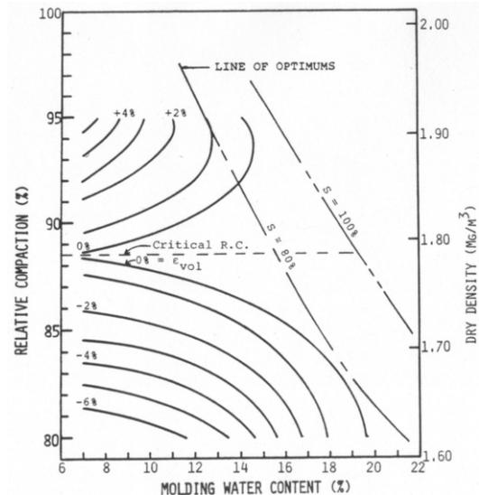
Fig. 3. Volume changes in a low plasticity clayey-sand fill (from Lawton et al., 1989)
