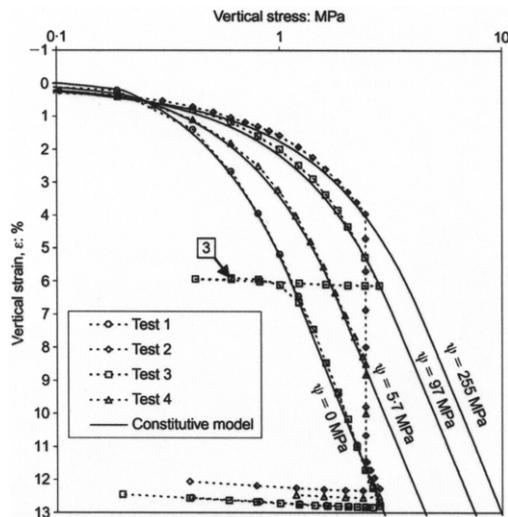
Figure 2. Effect of total suction on compressibility of rockfill (Oldecop & Alonso, 2003)
