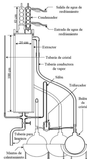
Figure 1. Extractor system used to simulate weathering of basalt (Maia et al., 2003)
