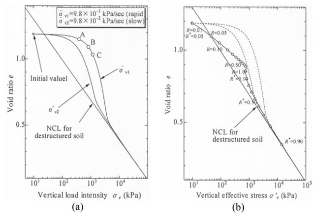
Figure 4. Breakdown of soil structure a) observed in 1-D experiments loaded as constant strain rate; b) numerical simulation of 1-D laboratory consolidation using Asaoka model (Asaoka et al., 2000)
