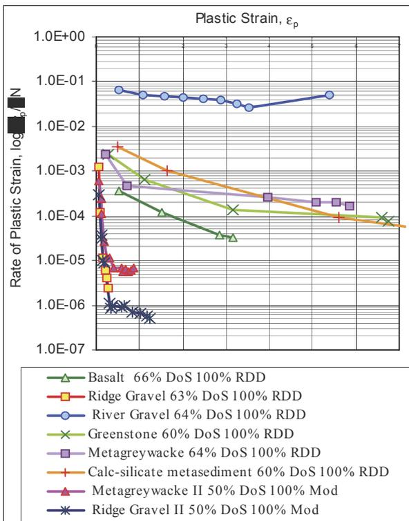
Figure 18. Rate of change of plastic strain vs plastic strain (Wijeyakulasuriya et al. 2005)
