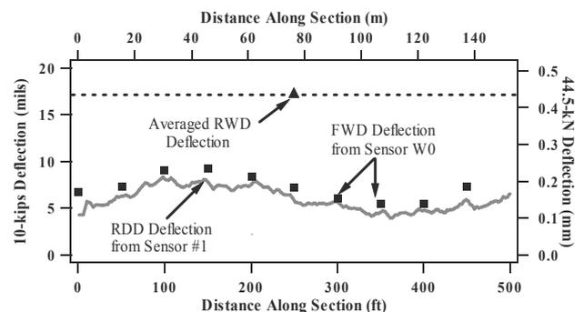
Figure 22. Comparison of results from different field loading tests (Lee and Stokoe and Bay, 2005)
