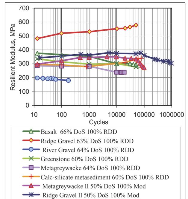
Figure 13. Unload-reload modulus as a function of number of cycles (Wijeyakulasuriya et al. 2005)
