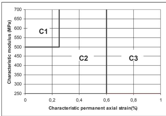
Figure 16. Classification for ranking mechanical behaviour of UGM (EN 13286-7)
