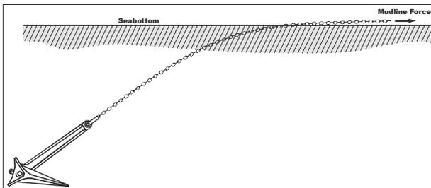
Figure 6. Schematic of drag anchor installation (Murff et al 2005)
