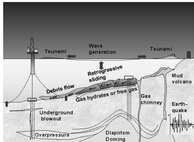
Figure 7. Offshore geohazards (Kvalstad personal communication 2002)
