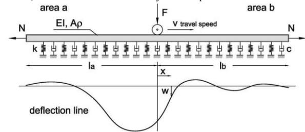
Figure 26. Sketch of a flexible beam resting on continuous spring-dashpot elements loaded by a moving single load (Koft and Adam, 2005).
