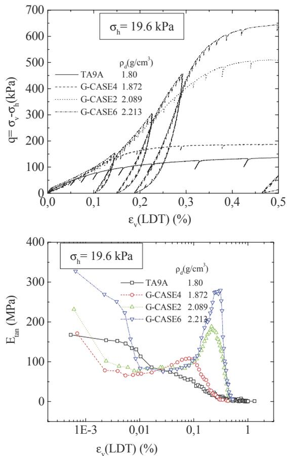
Figure 15. Relationships between (a) the deviator stress and the vertical strain – S shape; (b) tangent modulus and vertical strain, obtained from triaxial compression tests on moist Chiba gravel (Jiang et al, 1998 and Jiang and Kohata, 1998, cited by Tatsuoka et al., 1999)
