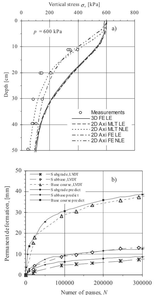
Figure 25. a) Vertical induced stress under the centre of a single tire as a function of depth (axial load: 160 kN; tire pressure: 600 kPa); b) Rutting prediction vs measurements of permanent deformation as a function of load repetition (Erlingsson 2005)
