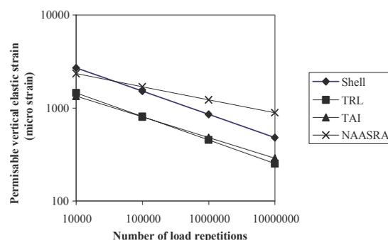
Figure 24. Different subgrade strain criteria
