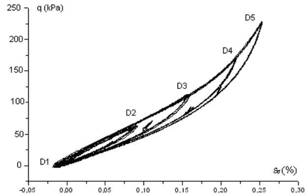
Figure 12. Closed loops of a granular material (granite aggregate 0/31.5mm) under unload-reload cycles after a preloading of 21.000 cycles with a constant deviator stress amplitude of 230 kPa and under a confining pressure of 40 kPa (Gomes Correia et al. 2005)
