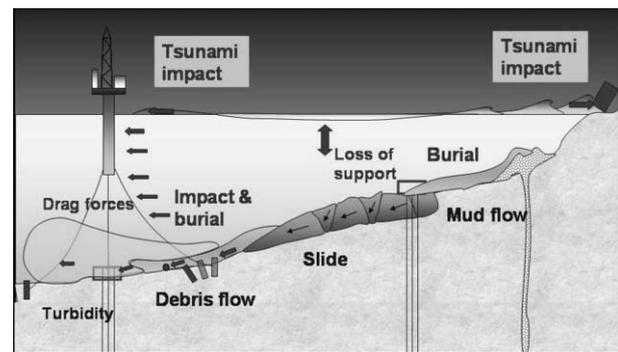
Figure 8. Impact of offshore geohazards on structures at sea and on land (Kvalstad personal communication 2002)
