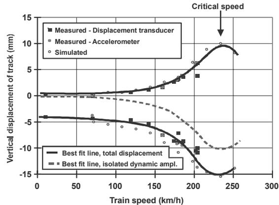
Figure 27. Peak upward and downward displacement of embankment at Ledsgård, Sweden, vs train speed. Values measured and simulated by VibTrain (Madshus and Kaynia, 2001, cited in Madshus, 2001)
