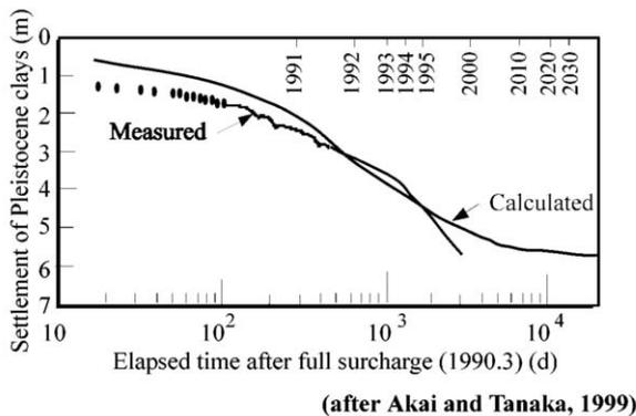
Figure 10. Analytical and measured settlement in a Pleistocene clay (Akai and Tanaka, 1999)
