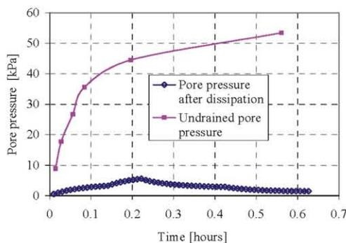
Figure 3. The prediction of excess pore pressure and pore pressure dissipation and the choice of ribs and drainage system resulted in important savings in the foundation costs (Hamre et al, 2005)
