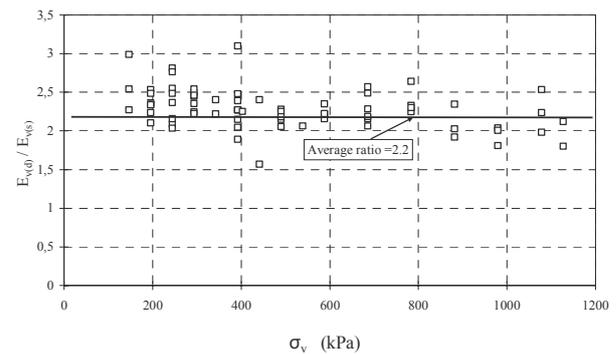
Figure 19. Ratio of the elastic Young's modulus obtained from the velocity in the wave transmission tests ( $E_{v(d)}$ ) to the value of ( $E_{v(s)}$ ) obtained from cyclic tests (Modoni et al., 1998)
