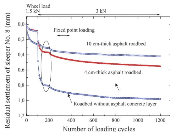
Figure 21. Permanent settlements of a sleeper (Momoya and Sekine, 2005)
