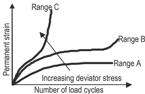
Figure 17. Different ranges of material deformation behaviour
