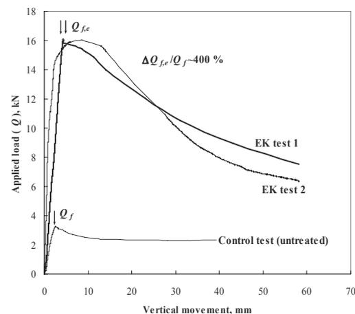
Figure 5. Increased pull-out resistance with electrokinetic treatment of clay (Micic and Lo, 2005)
