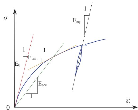
Figure 9. Modulus in a non linear stress-strain material behaviour
