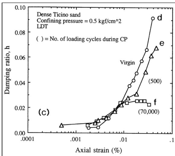
Figure 20. Influence of number of cycles in damping ratio of sands (Tatsuoka et al. (1995))
