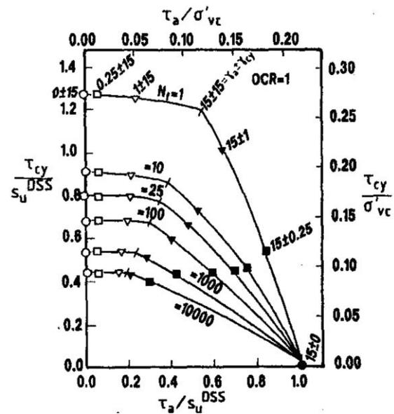
Figure 2. Number of cycles to failure,  $N_f$ , and shear strains at failure,  $\gamma_a = \gamma_{xy}$ , in simple shear tests (DSS) on Drammen clay with overconsolidation ratio of 1 (Andersen, 2004)
