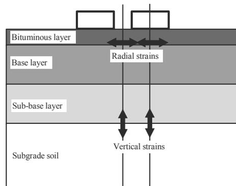
Figure 23. Sketch of a pavement structure and design criteria for two loading types
