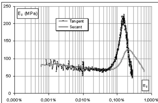
Figure 14. Tangent and secant moduli as a function of strain level for a very dense compacted granite 0/31.5 (Gomes Correia, 2004)
