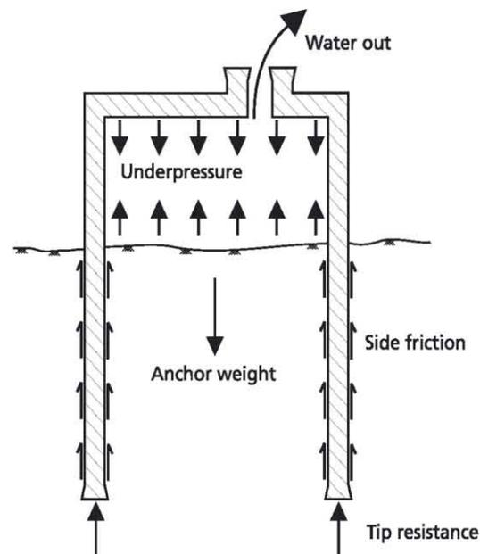
Figure 4. Skirted structure with the forces acting during penetration by underpressure (Andersen and Jostad, 1999)
