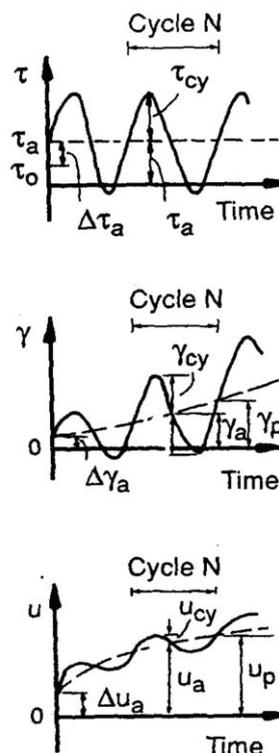
Figure 1. Shear stress ( $\tau$ ), shear strain ( $\gamma$ ) and pore pressure ( $u$ ) under cyclic loading ( $N$ = number of cycles, subscripts  $cy$ = cyclic,  $a$ =average,  $o$ =initial,  $p$ = permanent) (Andersen, 1991)
