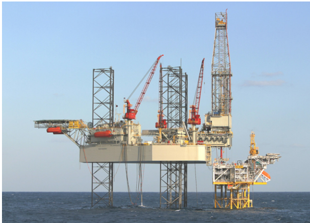
Figure 4. Photograph of mobile jackup rig (courtesy of Keppel Offshore and Marine Ltd.)
