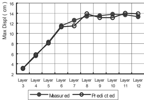
Figure 4. Comparison of the measured and predicted maximum displacements (Song et al.).
