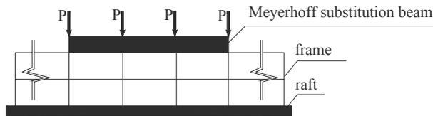
Figure 14: Simplified computation model (Gong et al.).
