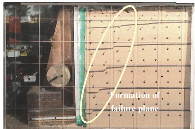
Figure 9. Formation of failure plane in the backfill after shaking at 350 gals (Koseki).
