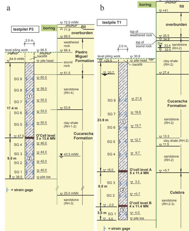
Figure 17. Single- and multi-level tests in the Cucaracha-Formation: test arrangement for test piles at axes P3 and T1 (Moormann and Humpf).
