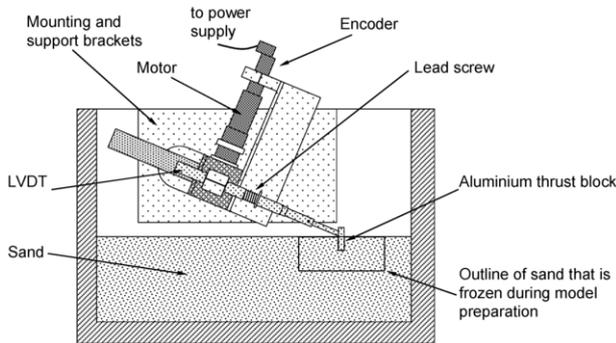
Figure 10. General set-up of apparatus (Goodey *et al.*).
