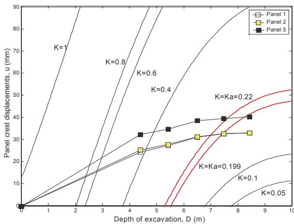
Figure 7. Superimposition of recorded thick panel displacements on predicted panel displacements (Chua and Bolton).
