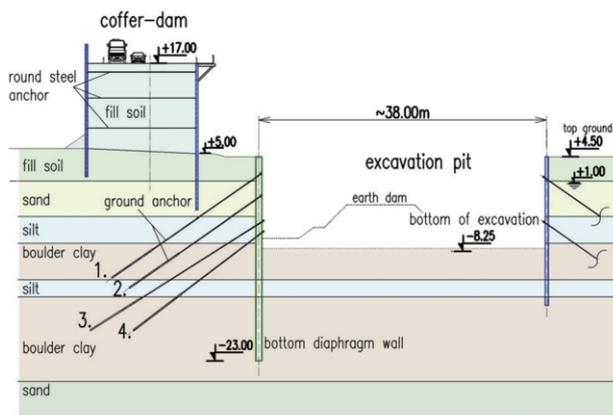
Figure 2. Cross section of the excavation after the re-design (Raithel *et al.*).
