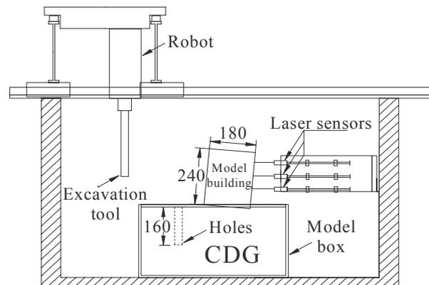
Figure 11. A sectional view of model package (unit: mm in model scale) (Ng *et al.*).
