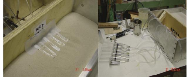
Figure 15. Test setup for simulating expanding tubes in the centrifuge: a) location empty tubes; b) syringe system for expanding tubes (Wichman and Allersma).
