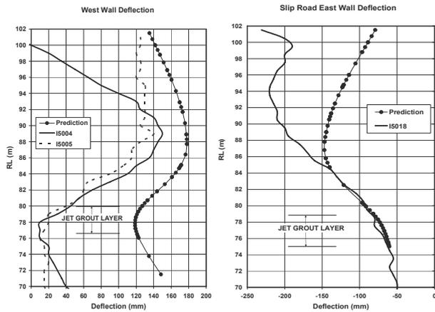
Figure 1. Measured and predicted (Class-A) sheet pile deflections (Hsi and Yu).
