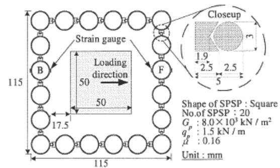
Figure 20. Plan view of the model foundation (Isobe and Kimura).
