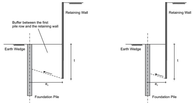
Figure 5. Section view through the earth wedge at different pile-wall-distances  $e_o$  (Katzenbach et al.).
