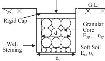
Figure 13. Short composite caisson foundation with granular core (Ali Jawaid and Madhav).
