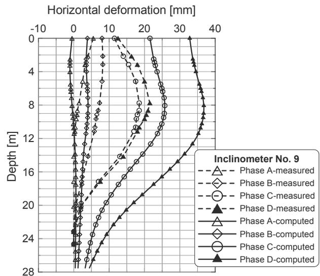
Figure 3. Measured versus computed deformations (Raithel *et al.*).
