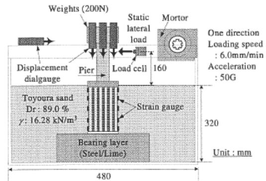
Figure 19. A cross-section of the model foundation (Isobe and Kimura).
