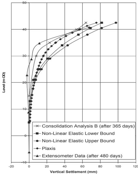
Figure 16. Predicted and observed settlement behaviour with depth (O'Brien et al.).
