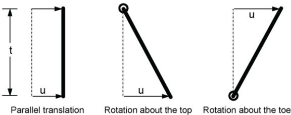
Figure 8. Types of the wall movement (Gebreselassie and Kempfert).
