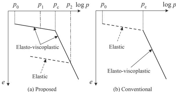
Figure 5. Compression model (after Mimura et al., 2005)
