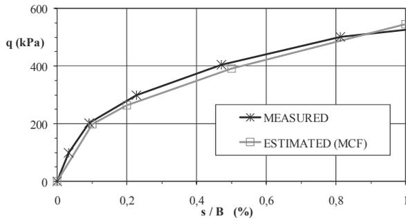
Figure 7. Computed and measured load-settlement curves.(after Bovolenta & Berardi, 2005)
