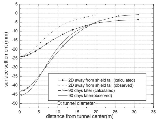
Figure 8. Comparison of calculated and in-situ measured surface settlements (after Huang et al., 2005)
