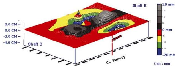
Fig. 10.3.4. Measured ground surface settlement after completion of the ESA construction under runway
