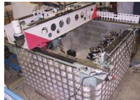
Fig. 10.1.1. The 4-axis robotic manipulator at HKUST (Ng et al. 2002b)
