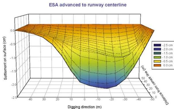
Fig. 10.3.3. 3-D Settlement prediction before construction
