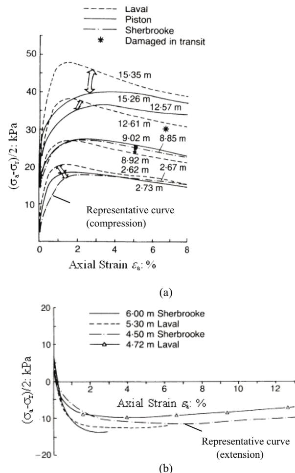
Figure 3 Soil stress-strain behaviour (after Hight et al., 1992) (a) CK<sub>U</sub> triaxial compression (b) CK<sub>U</sub> triaxial extension
