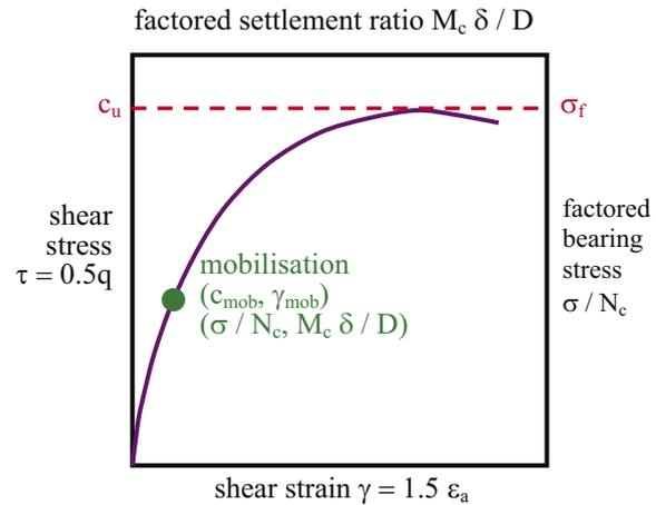
Figure 2 Bearing stress versus settlement for pad foundations
