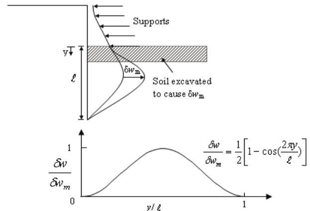
Figure 5 Incremental displacements in braced excavation (after O'Rourke 1993)
