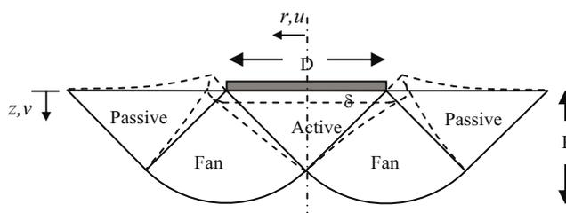
Figure 1 Plastic deformation mechanism for circular pad foundations
