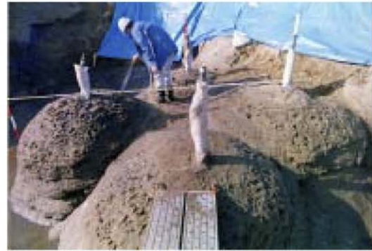
Photo 1 Improved soil excavated in a field test (Tsu-matsuzaka, Mie prefecture, 1998)
