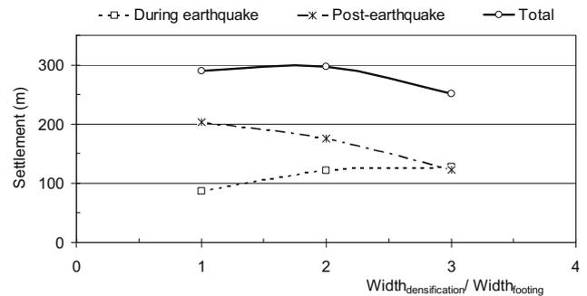
Figure 3. Settlements of the footing for different improvement widths
