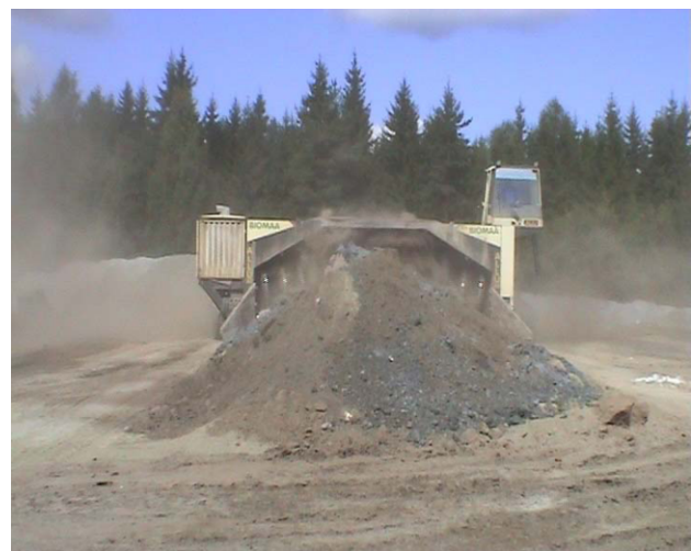
Figure 4: Stack mixer mixing fibre-ash (Kukkia Circlet, Pilot 2003)
