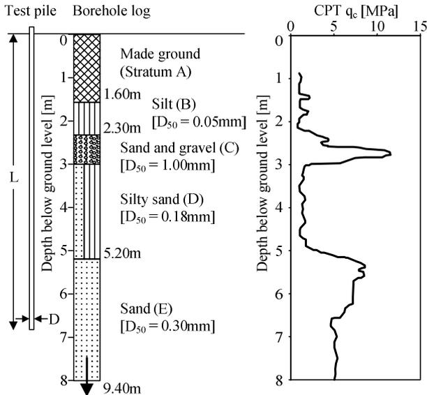
Figure 2. Ground conditions at test site
