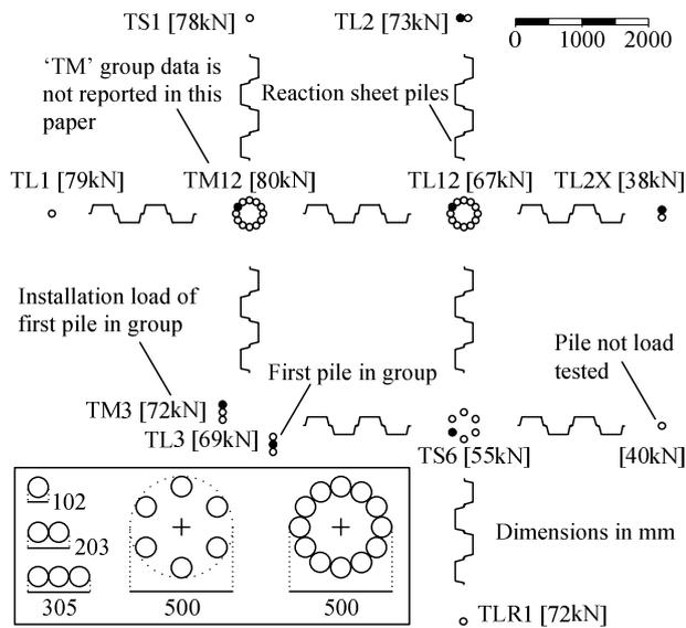
Figure 3. Arrangement of test piles
