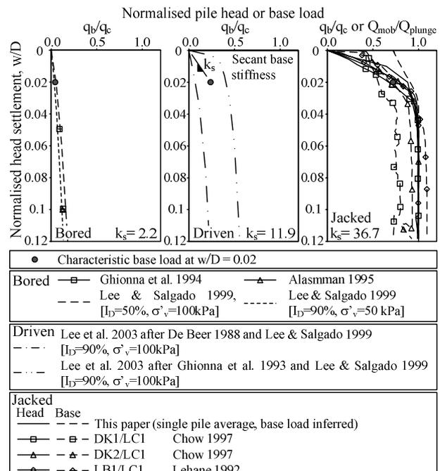
Figure 7. Relative stiffness of jacked, driven and bored piles
