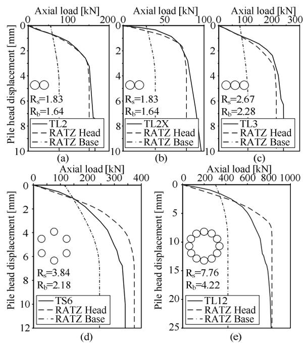
Figure 5. Load-settlement response of pile groups
