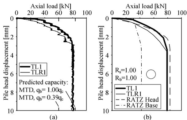
Figure 4. Load-settlement response of single piles
