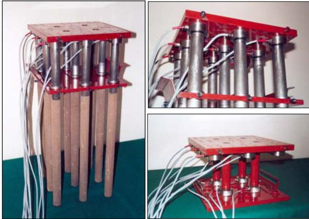
Figure 2 Piled raft foundation model.
