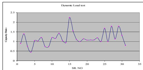
Figure 2. Ratio of safe test capacity & safe capacity from penetration resistance.
