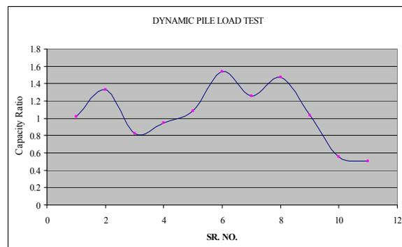
Figure 1. Ratio of safe test capacity & safe capacity from penetration resistance.
