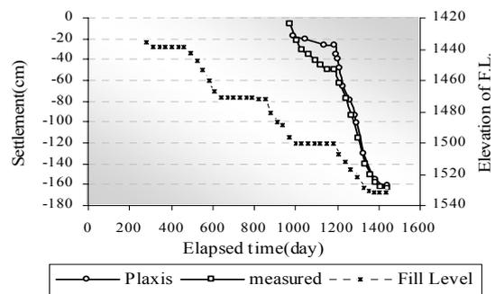
Figure 5. Settlement plate positioning (20<sup>th</sup>) in upstream of clay, elevation of installing: 1494.28
