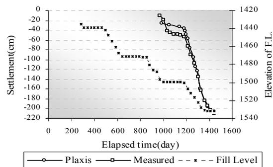
Figure 4. Settlement plate positioning (20<sup>th</sup>) in clay, elevation of installing: 1494.17
