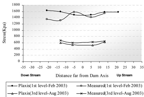
Figure 14. Vertical total stress in clay in 1<sup>st</sup> level, 1430 masl and 3<sup>rd</sup> level, 1483 masl, of installation
