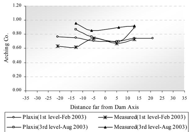
Figure 15. Arching coefficient in clay in 1<sup>st</sup> and 3<sup>rd</sup> level of installation
