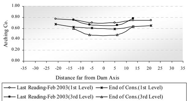
Figure 16. Predicted arching coefficient in clay in 1<sup>st</sup> and 3<sup>rd</sup> level of installation
