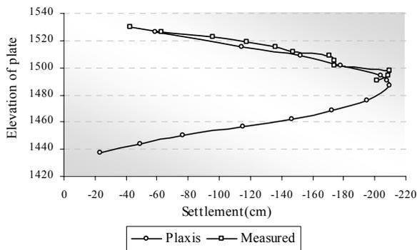
Figure 7. Settlement plates positioning in clay (Feb 2003)
