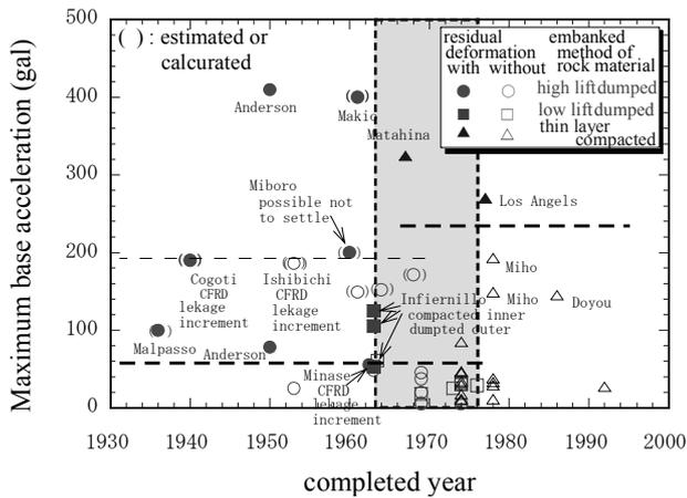
Figure.2 Relation between Maximum Base Acceleration and Completed Year with and without Seismic Damage (Okamoto T., 2004)
