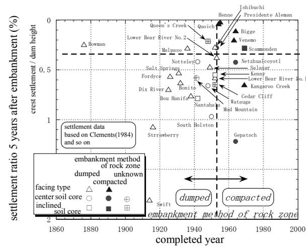
Figure.3 Dependency of Embankment Method on Settlement Ratio after Completed Embankment for Japanese Dams (Okamoto T., 2004)
