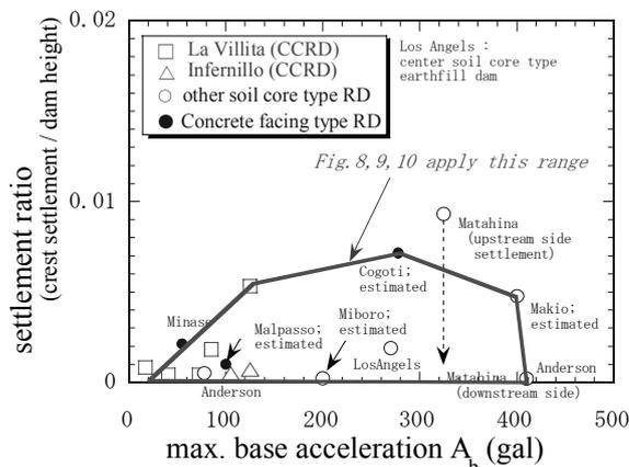
Figure.1 Residual Crest Settlement and Max. Base Acceleration of In-situ Observation (Okamoto T., 1999)
