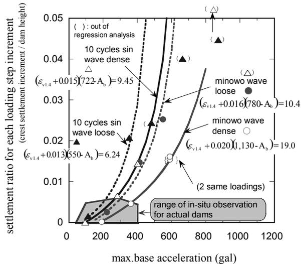
Figure.8 Incremental Crest Settlement and Max. Base Acceleration by Centrifuge Test (Okamoto et al. :2004)
