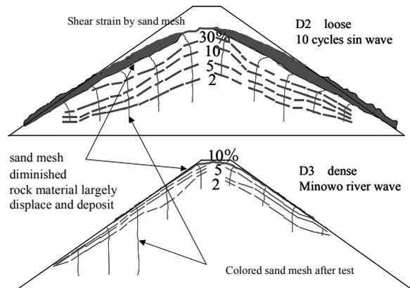
Figure.6 Final Residual Deformation and Shear Strain by centrifuge shaking table test (Okamoto et al. : 2004)
