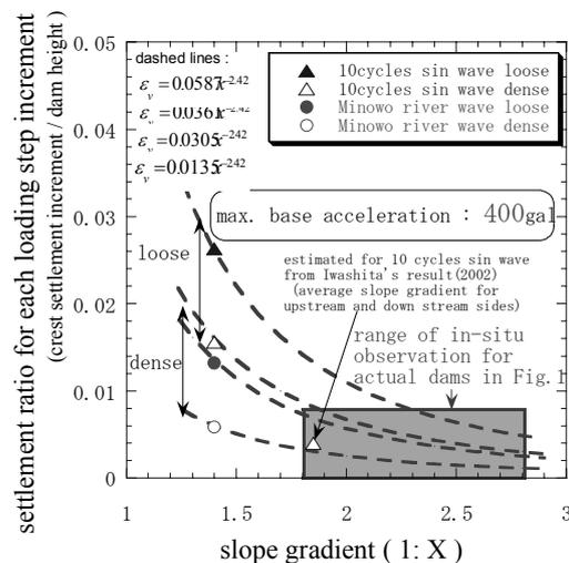
Figure.9 Effect of Slope Gradient on Residual Settlement (Max. Base Acceleration 200gal)
