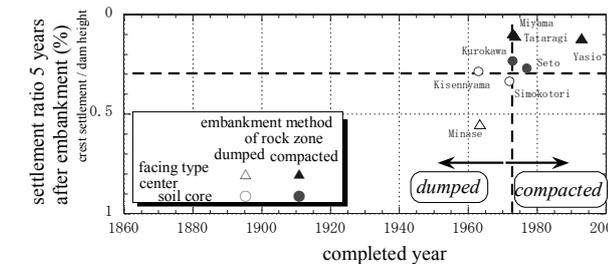
Figure.4 Dependency of Embankment Method on Settlement Ratio after Completed Embankment except Japanese Dams (Okamoto T., 2000)
