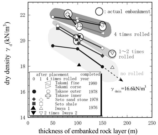
Figure.5 Density of Rock Zone by In-situ Compaction Test (Okamoto T., 2004)
