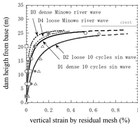
Figure.7 Vertical Strain along Center Axis after Shaking by Okamoto et al. (2004)
