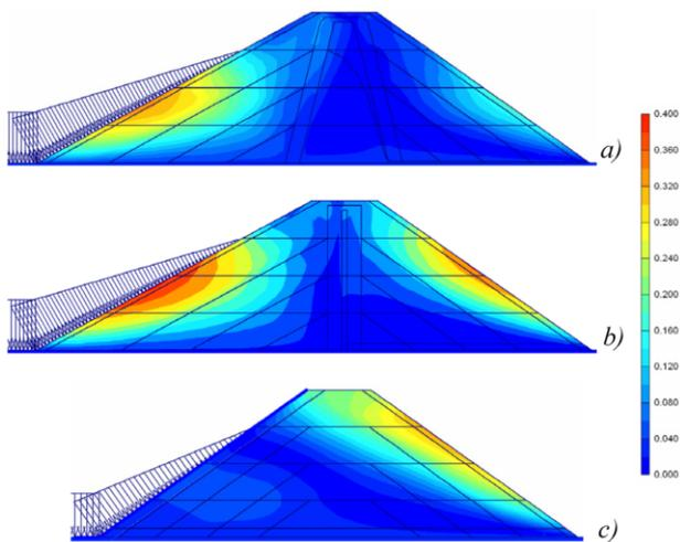
Figure 9. Permanent displacement after applying seismic load, coloured scale in meters. a) Rockfill dam with a loessoidal core. b) Rockfill dam with an asphaltic core. c) Rockfill dam with a concrete face.
