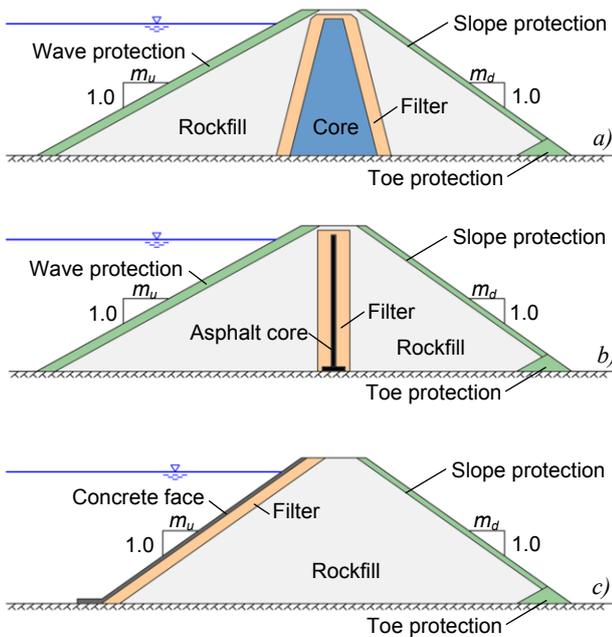
Figure 1. Typical cross sections for the proposed dams in the Lower Thjorsa River. *a)* Rockfill dam with a central core of loessoidal soil. *b)* Rockfill dam with a central core of asphaltic concrete. *c)* Rockfill dam with an upstream concrete face.
