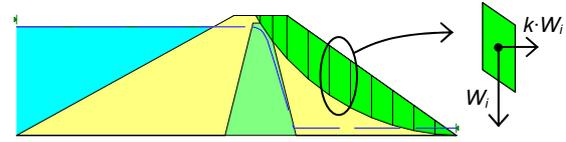
Figure 6. A typical slip surface in the downstream slope of a dam section with a central soil core. A horizontal pseudo static seismic force equal to  $k \cdot W_i$  is applied to each slice, where  $W_i$  is its weight.
