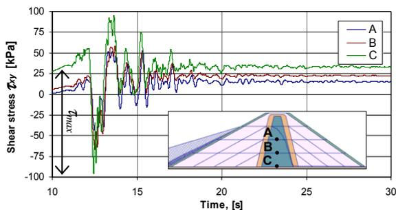
Figure 10. Shear stress development in the core material during earthquake loading, corresponding to the last time series in Figure 5.
