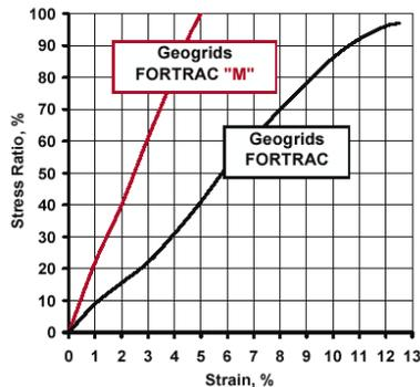
Figure 12. A 63 Selby Bypass typical normalized stress-strain curves for the geogrids used
