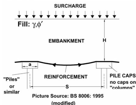
Figure 1. General idea of reinforced embankments on piles
