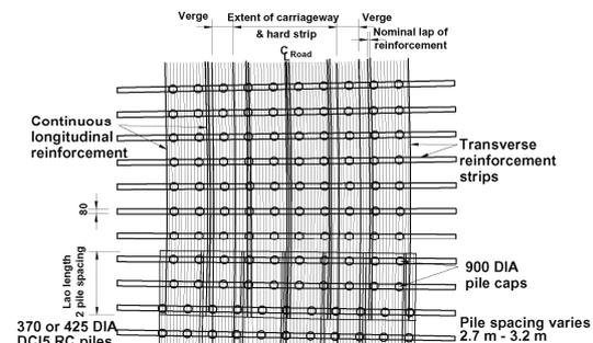
Figure 11. A 63 Selby Bypass: typical layout of reinforcement
