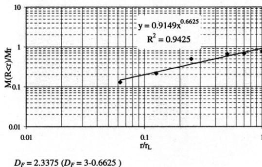
Figure 2. Typical plot of sieve analysis results to obtain  $D_F$  at a normal stress = 1374.3 kPa.
