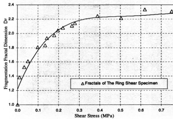
Figure 3. Fragmentation fractal dimension values for sand subjected to crushing in ring shear test.
