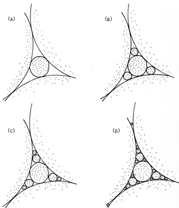
Figure 5. A pore being filled by a fractal soil.
