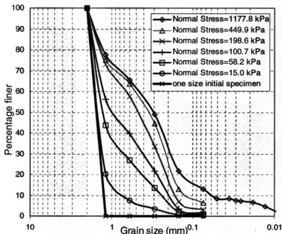
Figure 1. Grain size distribution of sand crushed in the ring shear apparatus.
