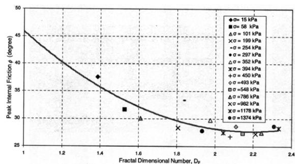
Figure 6. Relationship between friction angle,  $\phi$ , and the fragmentation fractal dimension  $D_F$ .
