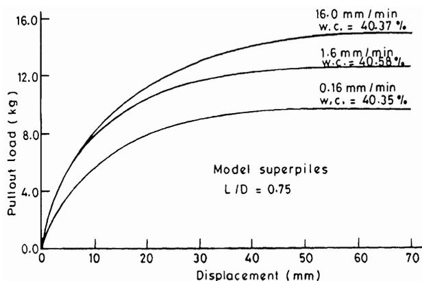
Figure 3. Behavior of model superpiles during static pullout
