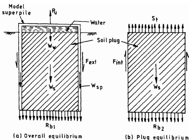
Figure 2. Equilibrium of model superpiles anchors in laboratory tests
