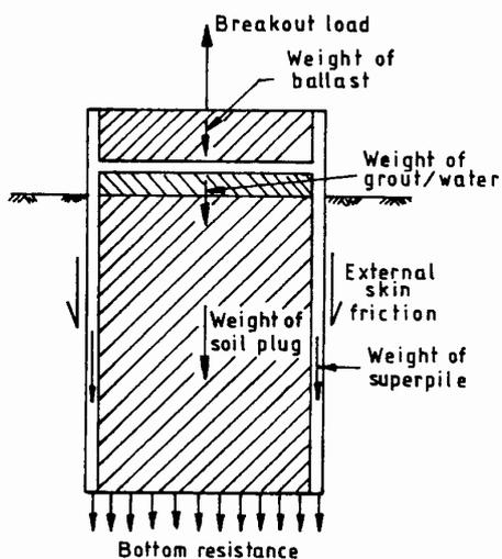
Figure 1. Components of breakout load for a superpile anchor
