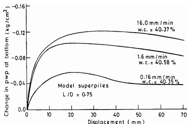
Figure 5. Variation of pore water pressures beneath the base of model superpiles
