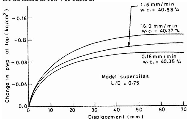
Figure 4. Variation of pore water pressures above soil plug in model superpiles during static pullout
