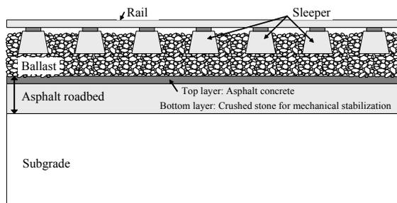
Figure 1. Typical cross-section of railway asphalt roadbed.
