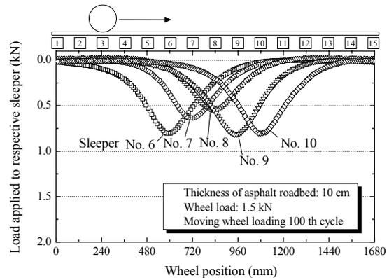
Figure 5. Vertical load applied to respective sleepers.
