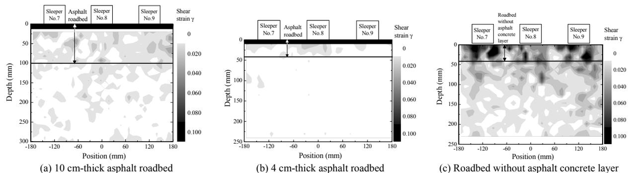
Figure 9. Residual shear strain in the roadbed and sugrade at the end of the moving-wheel loading tests.
