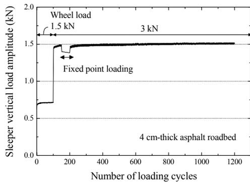
Figure 10. Sleeper No. 8 vertical load amplitude.
