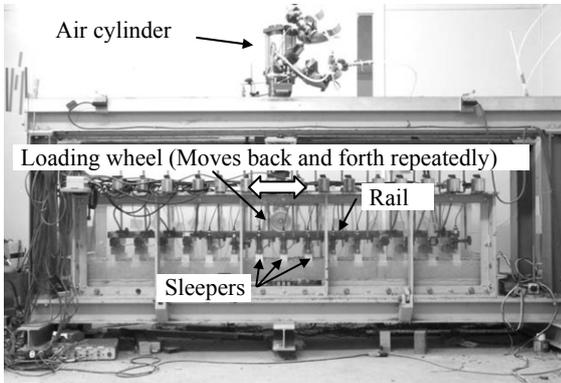
Figure 2. Moving-wheel loading test apparatus.
