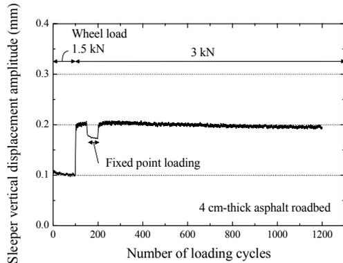
Figure 11. Sleeper No. 8 vertical displacement amplitude.
