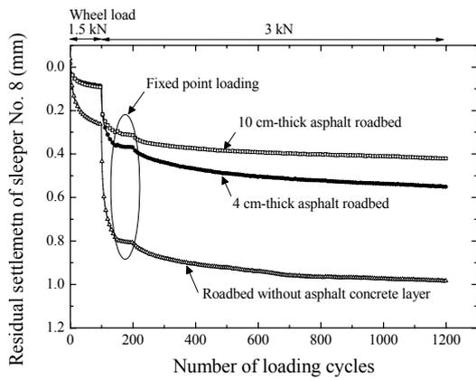
Figure 7. Residual settlement of sleeper No. 8.
