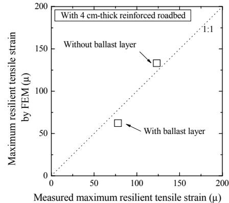
Figure 13. The maximum resilient strain of asphalt concrete layer in the scale model test and FEM, with and without ballast layer.
