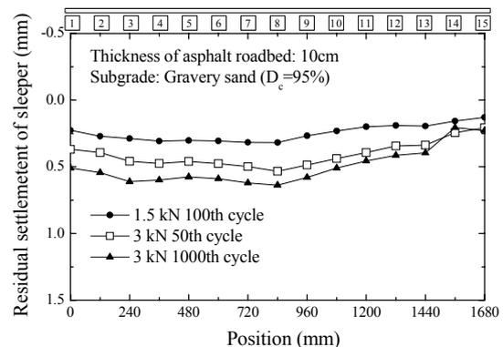
Figure 6. Residual settlement of respective sleepers.
