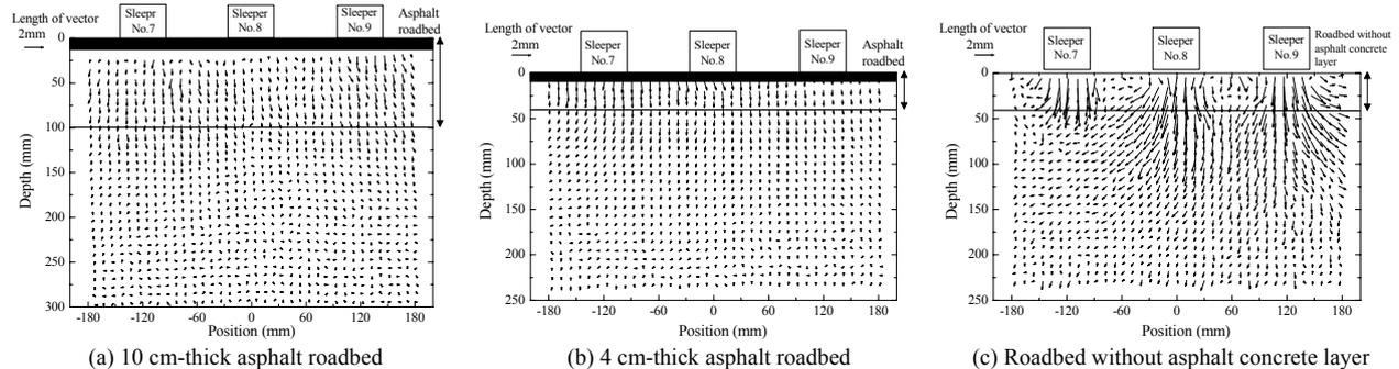
Figure 8. Residual deformation in the roadbed and sugrade at the end of the moving-wheel loading tests.
