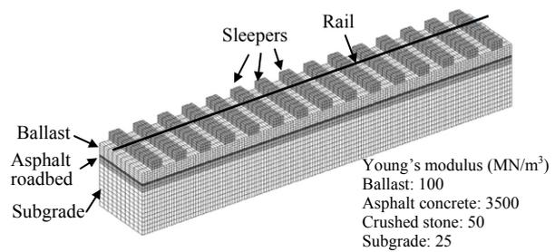
Figure 12. Three dimensional FEM model.
