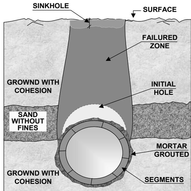
Figure 3. final dorsal instability (cross section).
