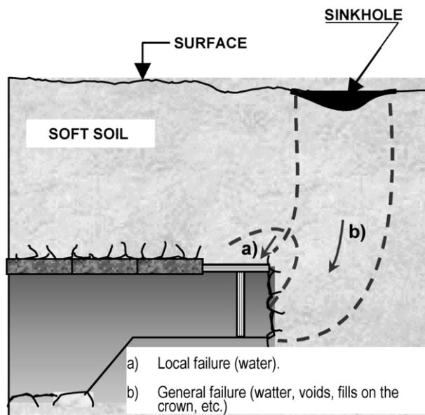
Figure 1. Lay-out of frontal tunnel instability.
