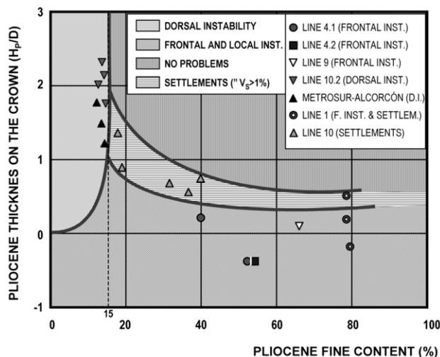
Figure 11. Instability problems criteria for the Madrid Ground and E.P.B. excavation.
