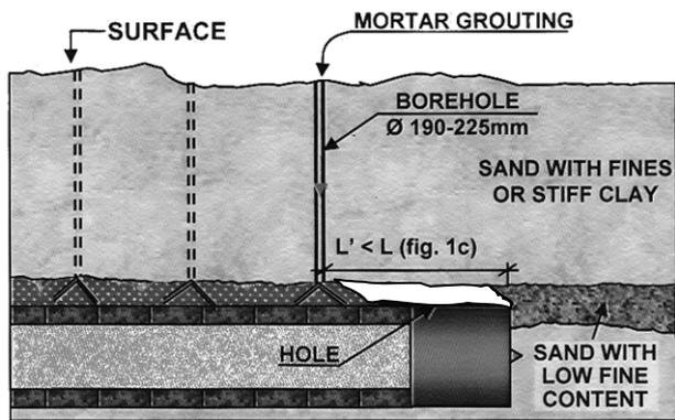
Figure 9. Example of the ground treatment from the surface with mortar (Arnaiz and Melis, 2003).
