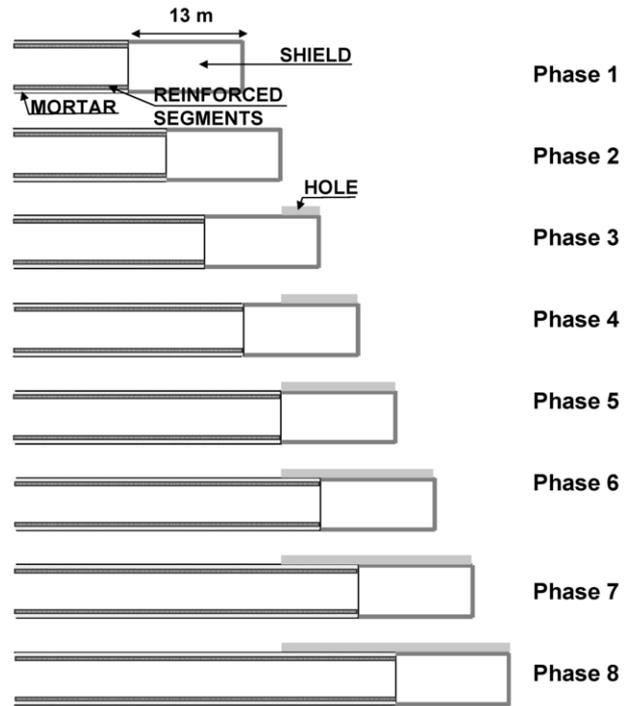
Figure 7. Theoretical simulation of the tunnel advance and dorsal instability (PLAXID-3D analysis).
