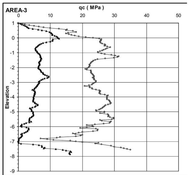
Figure 5. CPTs performed BEFORE and AFTER densification of Hydraulic Fills at three different areas
