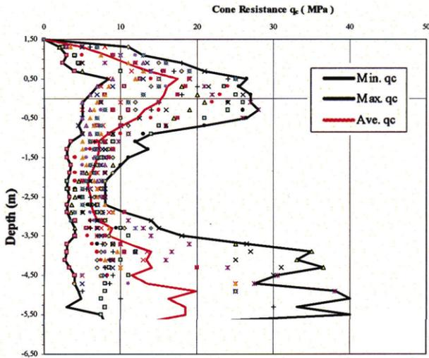
Figure 2. CPTU tests performed BEFORE Densification of Sand Fills
