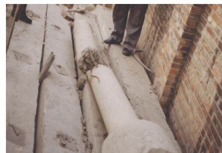
Figure 10. Crush of mini pile exhumed after loading test
