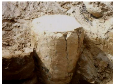
Figure 5. DMM column head after single DMM column loading test
