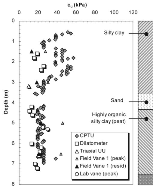
Figure 2. Undrained shear strength profile of the natural soil at the site.
