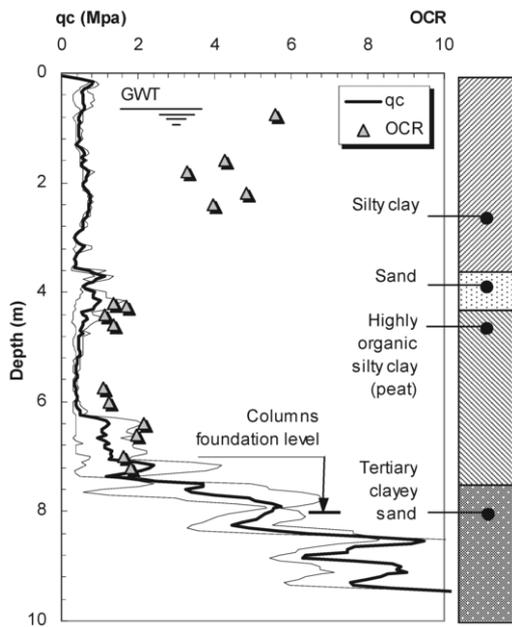
Figure 1. Natural soil profile at the test site.
