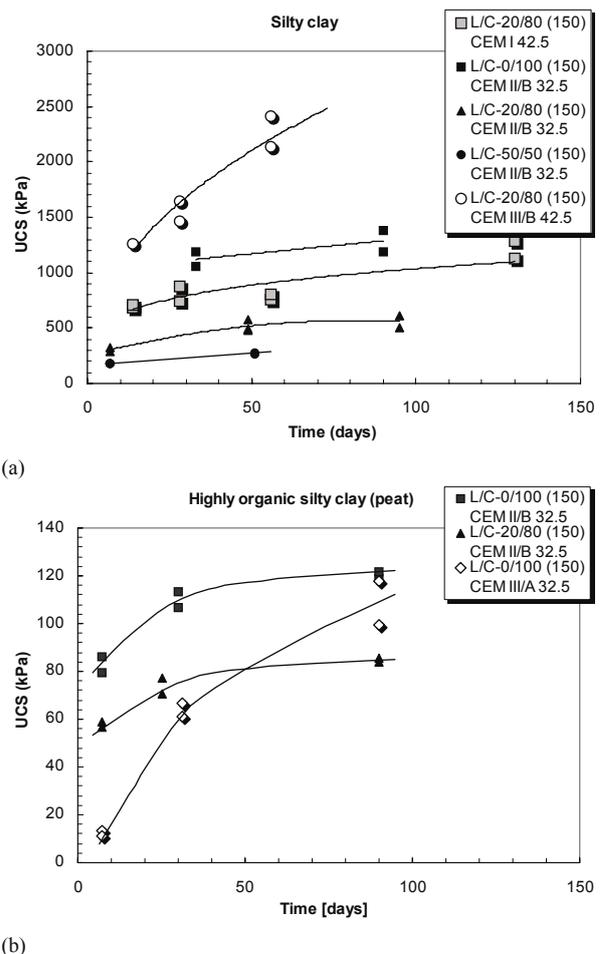
Figure 3. UCS of (a) silty clay and (b) highly organic silty clay, mixed in the laboratory with a binder dosage of 150 kg/m<sup>3</sup>.
