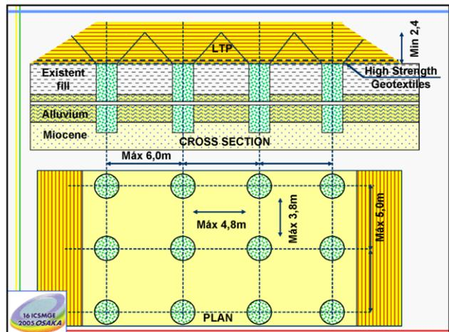
Figure 10. Road platform: transversal cross section and plan.
