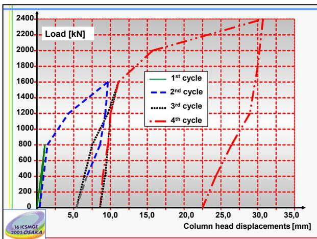
Figure 4. Full scale vertical load test: load vs. head displacements.
