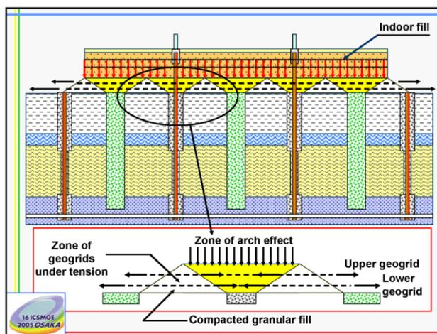
Figure 2. LTP under an industrial building: arch effect.
