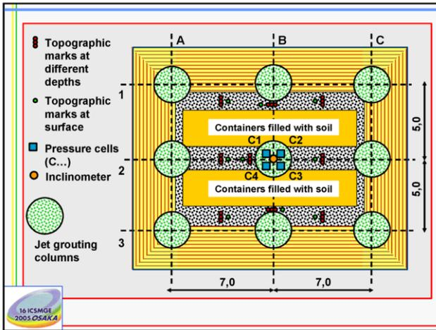
Figure 6. Static railway full scale load test: plan and monitoring.
