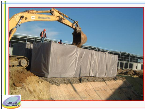
Figure 7. Static railway full scale load test: filling of containers.
