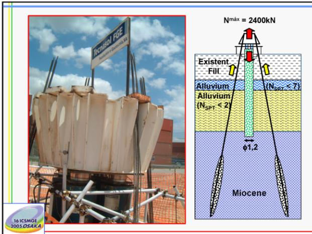
Figure 3. Full scale vertical load test: load and reaction device.
