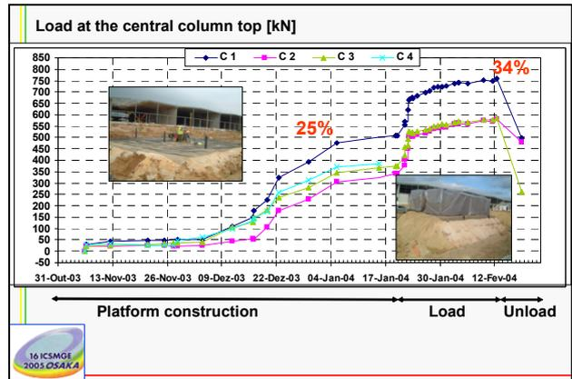
Figure 9. Static railway full scale load test: load at the central column.
