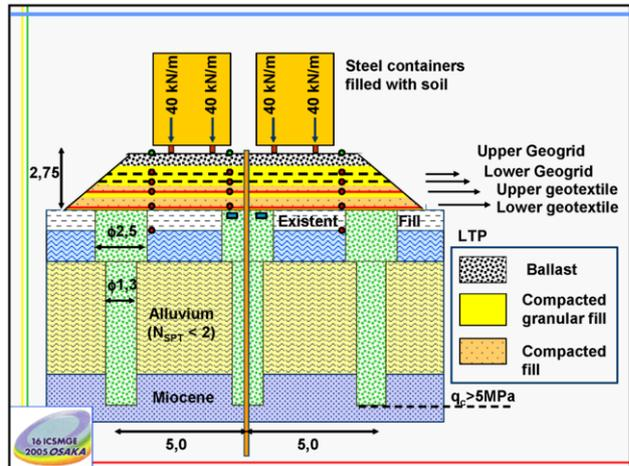
Figure 5. Static railway full scale load test: transversal cross section.
