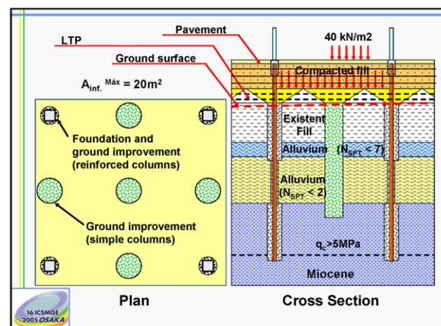
Figure 1. LTP under an industrial building: columns mesh.
