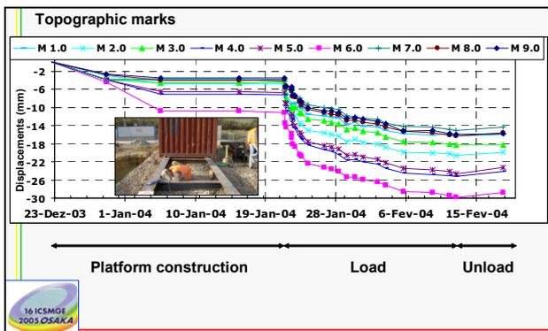
Figure 8. Static railway full scale load test: load - surface displacements.
