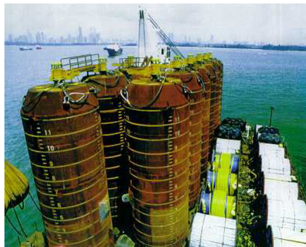
Figure 6.3 Suction caissons for the Laminaria field in the Timor Sea.
