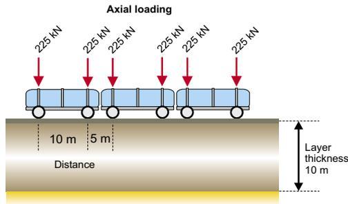
Figure 10. Numerical calculated freight wagons.
