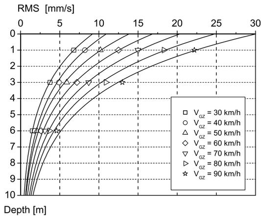
Figure 5. RMS vs. depth for test track TS0.
