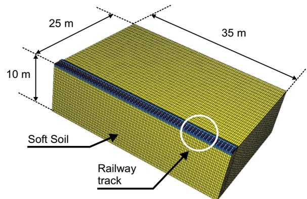
Figure 8. 3D-Finite Element Model.
