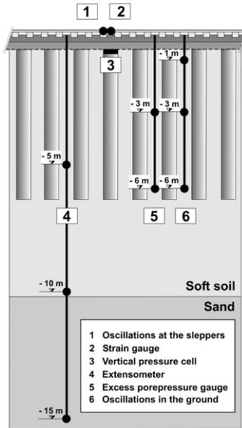
Figure 2. Layout of the measurement devices (example: TS1).
