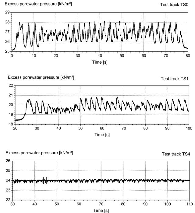
Figure 4. Excess porewater pressure measurements in TS0, TS1 and TS4.
