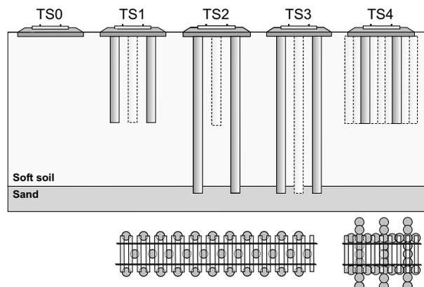
Figure 1. Column arrangement installed in the test field.
