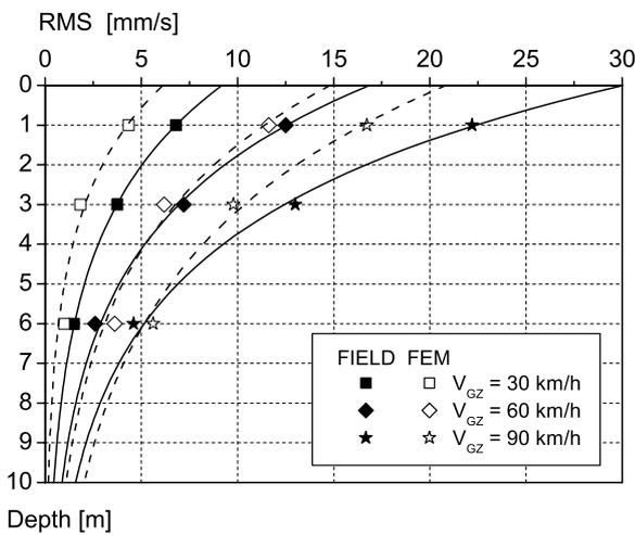
Figure 11. RMS, measurement vs. FEM, TS0.
