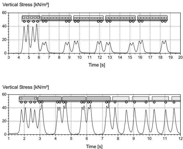
Figure 3. Vertical stress for passenger and freight train.
