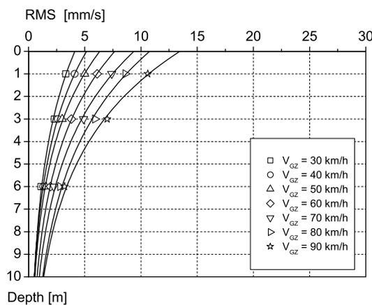
Figure 6. RMS vs. depth for test track TS1.
