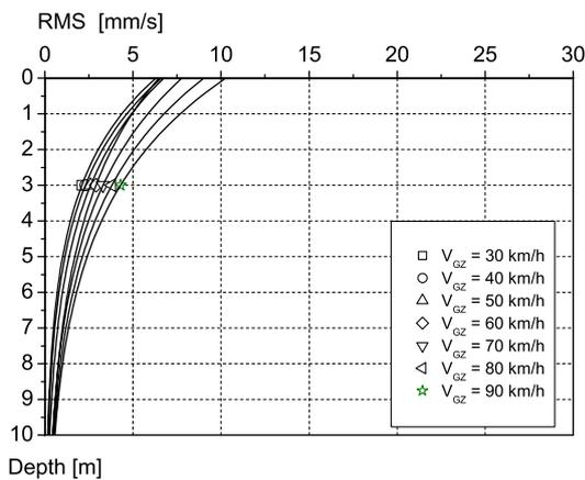
Figure 7. RMS vs. depth for test track TS4.
