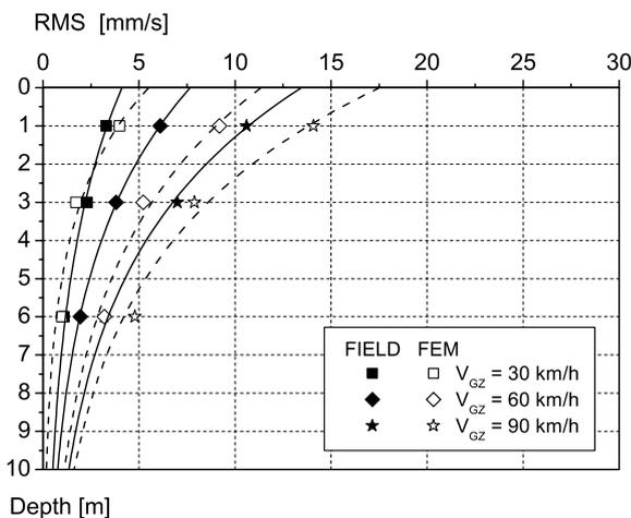
Figure 12. RMS, measurement vs. FEM, TS1.
