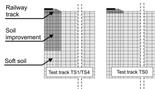
Figure 9. 3D-Finite Element Model (cross section).
