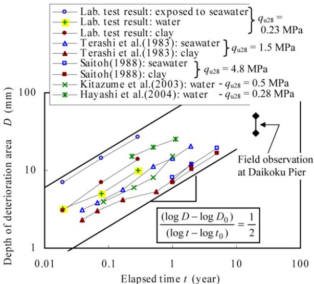
Figure 9. Progress of the deterioration area with time.
