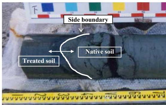
Photo 1. The core sample of Bor. No. 3 at the side boundary.
