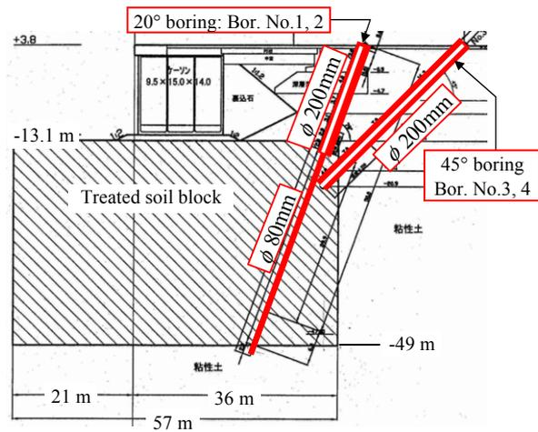
Figure 1. Cross section of the improved ground and borings.
