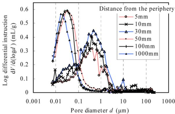
Figure 7. Pore size distributions of the treated soil.
