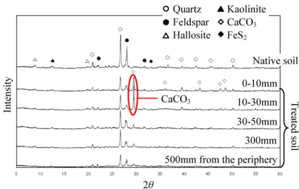
Figure 8. X-ray diffraction patterns from treated and native soil.
