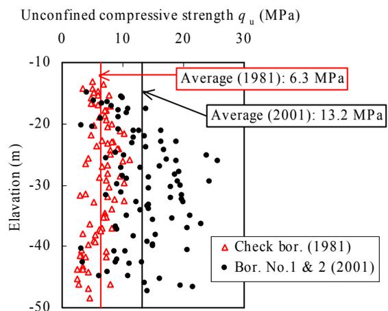
Figure 3. Strength distributions with elevation.
