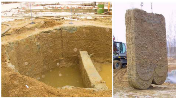
Fig 7: Wall details and exhumed test panel
