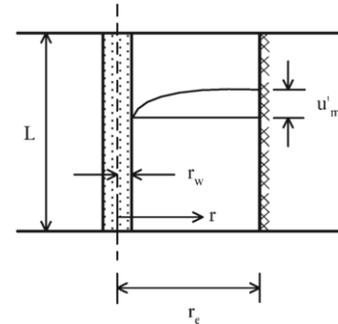
Fig. 2 Excess porewater pressure distribution for vertical compression and radial flow into vertical drain
