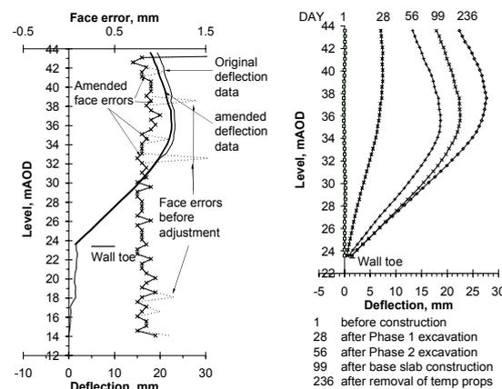
Figure 2 – (a) Analysis of inclinometer face errors (b) Wall profiles measured with the inclinometer during excavation in front of the wall
