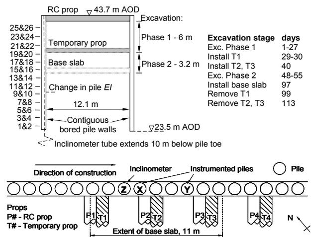
Figure 1 – Elevation and plan showing construction sequence and pile and prop locations
