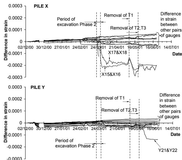
Figure 3 – Difference in strain measured in pairs of strain gauges over the period of construction
