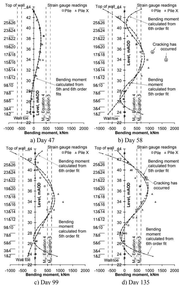
Figure 4 – Bending moments calculated: before (a) and after (b) excavation Phase 2 and before (c) and after (d) temporary prop removal
