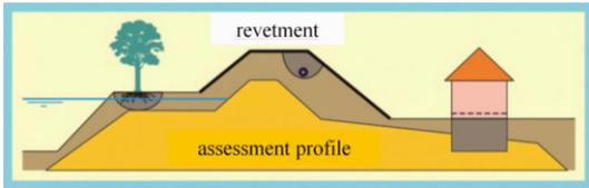
Figure 1. Non-water retaining objects in a dike (MIM, 2007)
