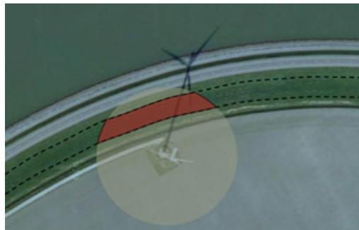
**Figure 2.** Estimation of the probability of an impact of a falling wind turbine object in dike)
